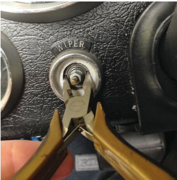
Figure 16 – Remove Switch Nut
