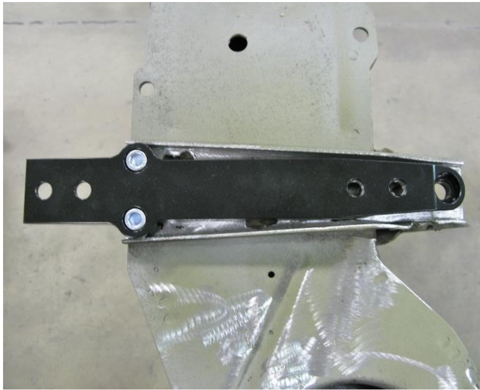
Figure 4 – Position Cradle Crossmember Adapter Plates
