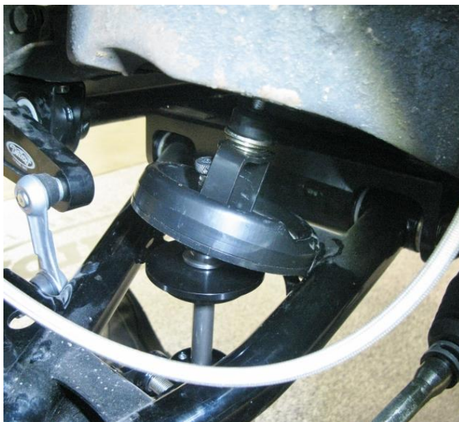
Figure 30 – Install Coilover Shock Assembly
