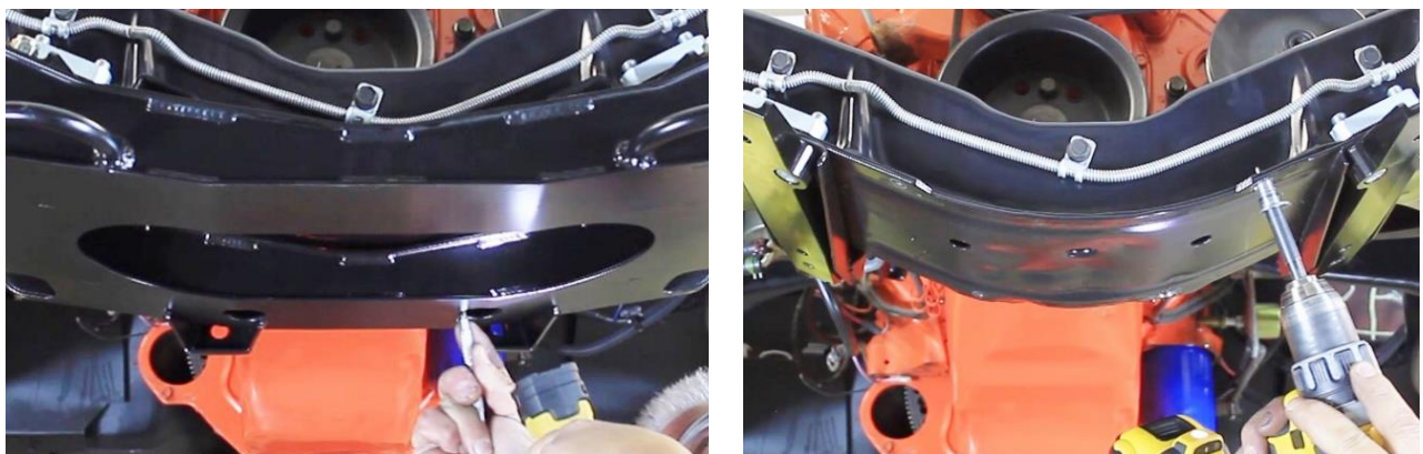
Figure 7 – Locate & Drill Mounting Holes
