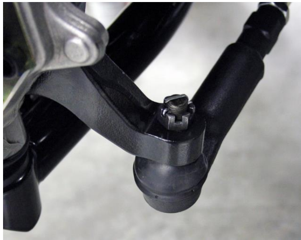
Figure 23 – Install Tie Rod Ends to Steering Arms
