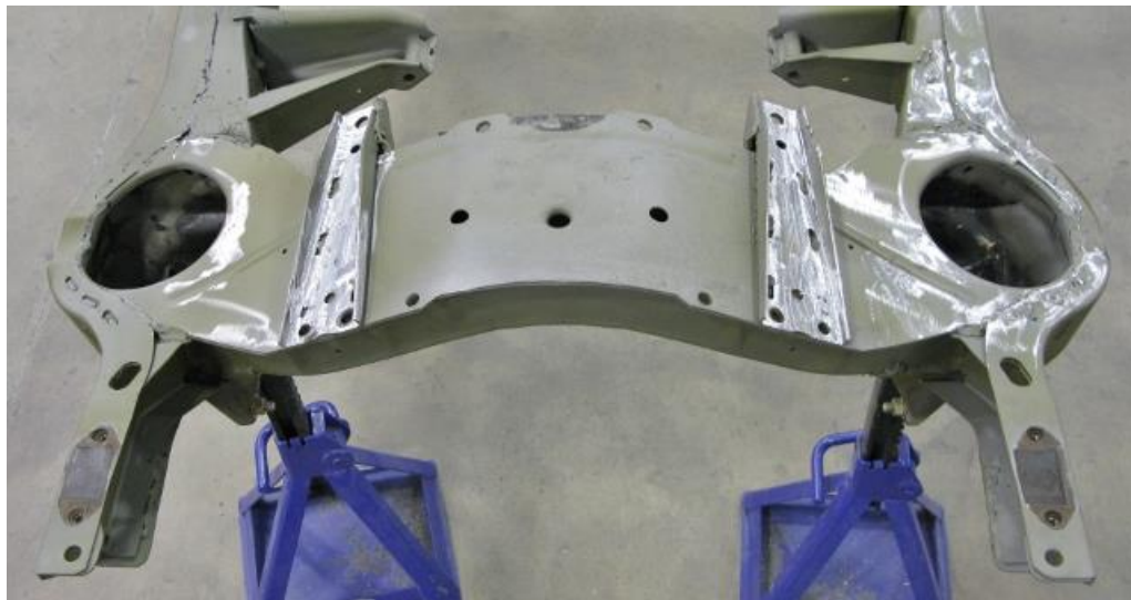
Figure 3 – Grind Lower Control Arm brackets
