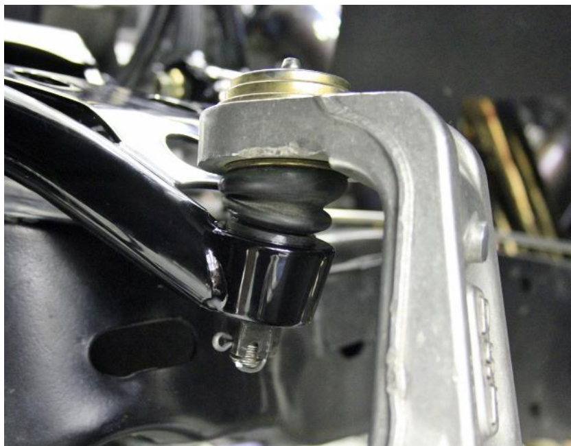
Figure 21 – Install Upper Ball Joint
