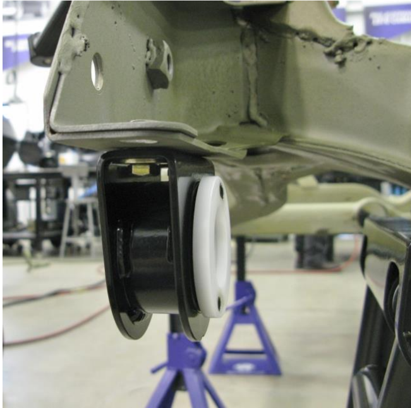
Figure 16 – Install Sway Bar Bracket Assembly
