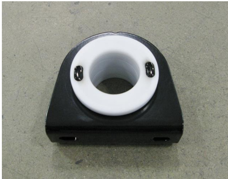
Figure 15 – Install Sway Bar Composite Bushings
