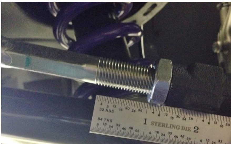
Figure 11 – Install the Tie Rod Ends
