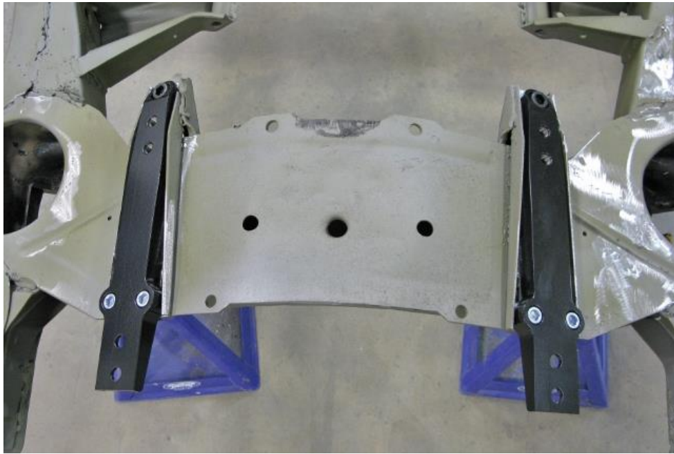
Figure 6 – Install Adapter Plates to Crossmember
