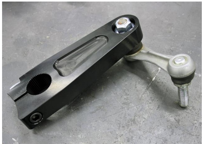
Figure 19 – Install Endlinks to the Sway Bar Arms
