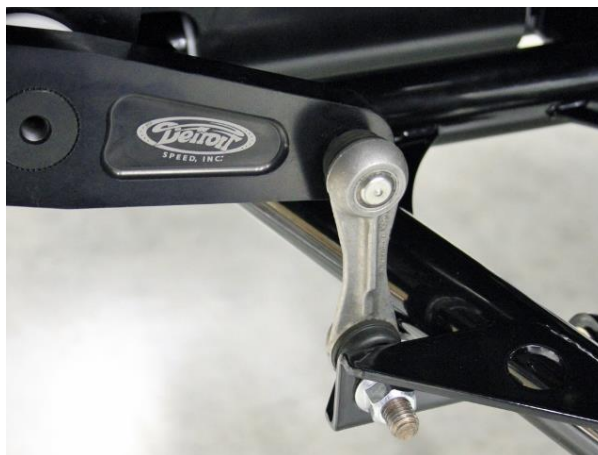
Figure 24 – Install the Sway Bar Endlinks to the Lower Control Arms
