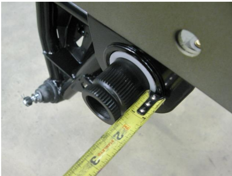
Figure 17 – Install Splined Sway Bar
