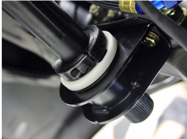
Figure 18 – Install Sway Bar Split Lock Collars
