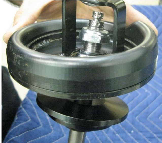
Figure 29 – Assemble Coilover Upper Mount
