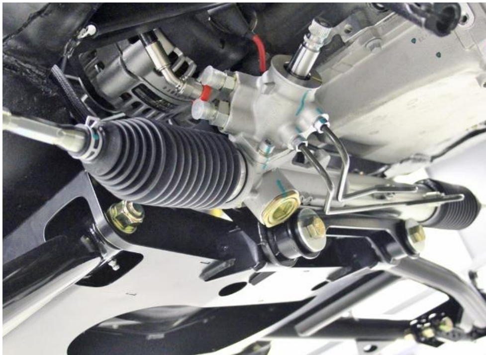
Figure 23 – Install Rack & Pinion
