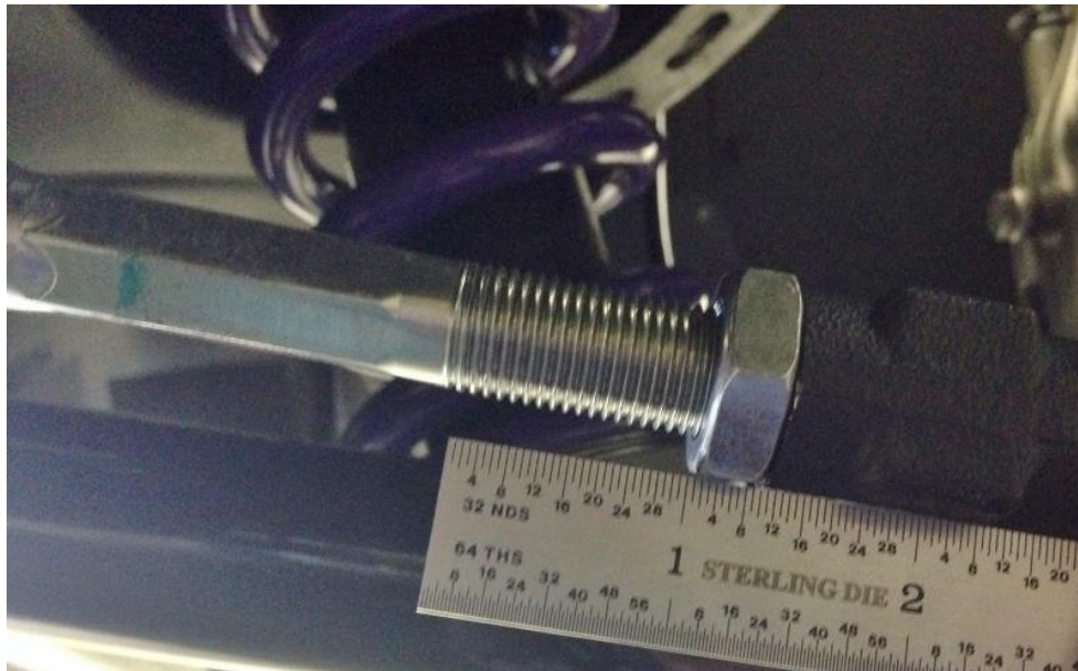
Figure 22 – Install the Tie Rod Ends
