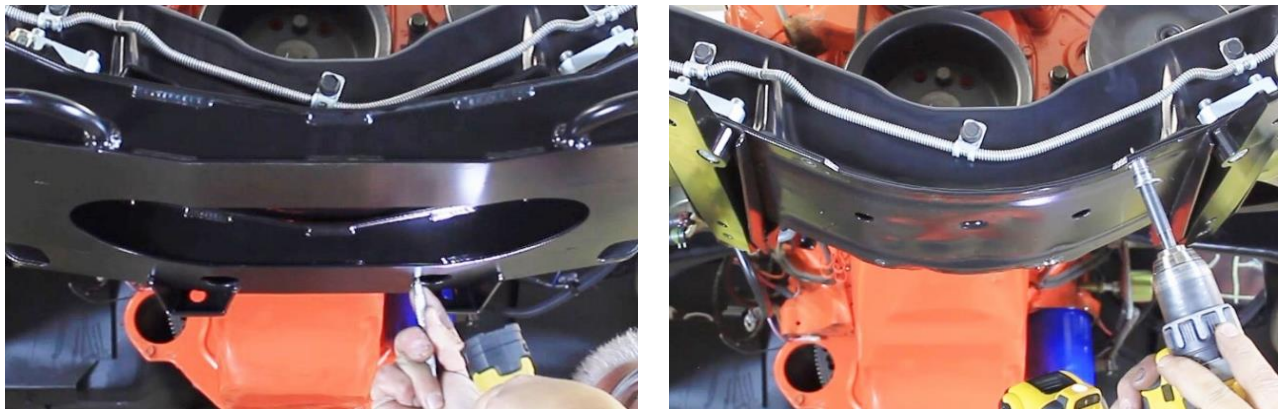
Figure 18 - Locate & Drill Mounting Holes
