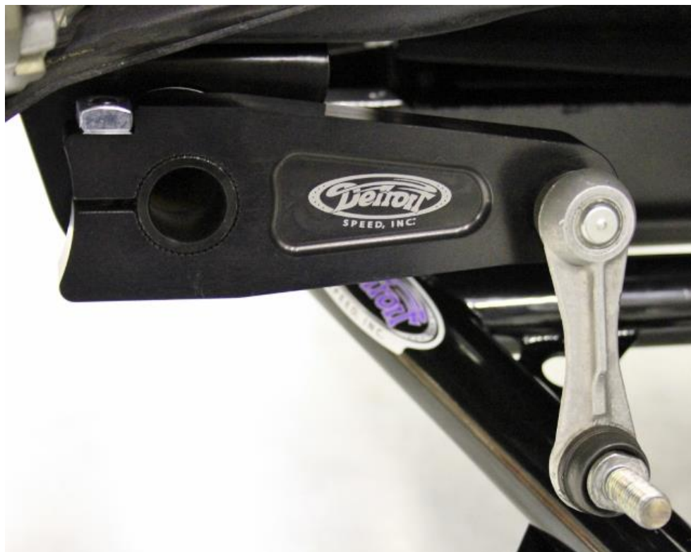
Figure 31 – Driver Side Sway Bar Arm
