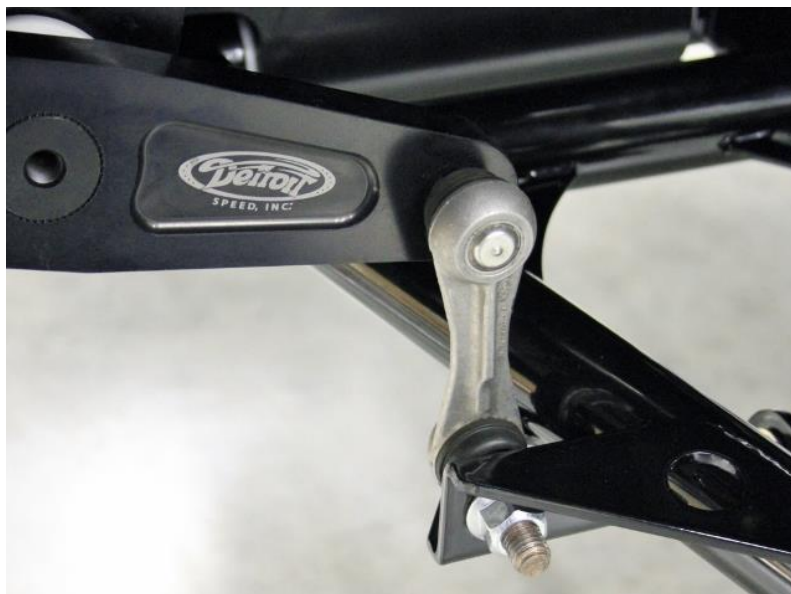
Figure 35 - Install the Sway Bar Endlinks to the Lower Control Arms
