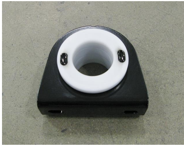
Figure 26 – Install Sway Bar Composite Bushings
