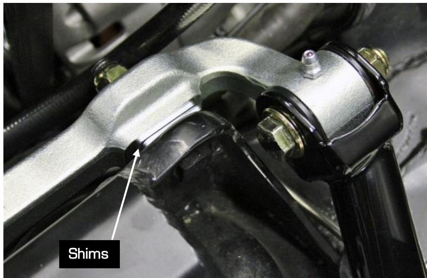
Figure 25 - Install 1/8" Shims
