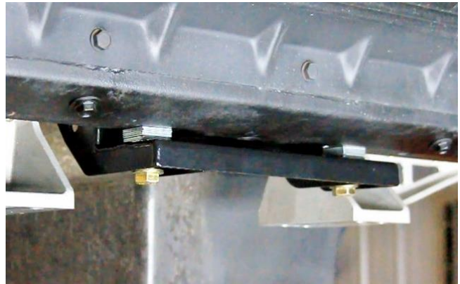
Figure 82 - Install Fasteners & Slotted Shims
