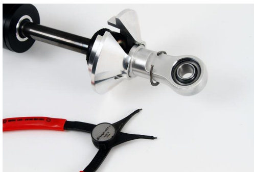
Figure 106 – Removing the Snap Ring
