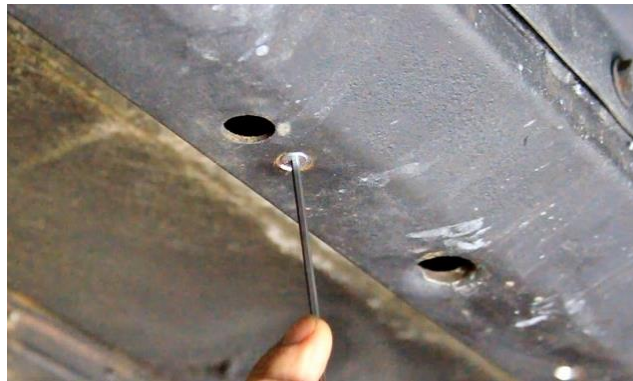
Figure 34 – Drill & Chamfer Holes
