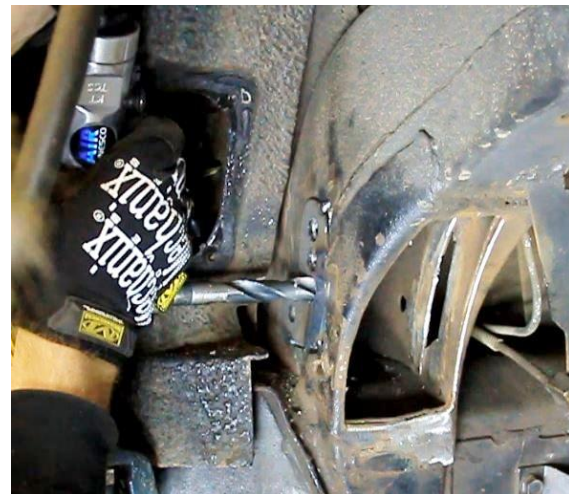
Figure 13 – Drill Trailing Link Holes
