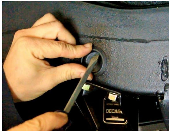
Figure 114 – Install Recessed Plug
