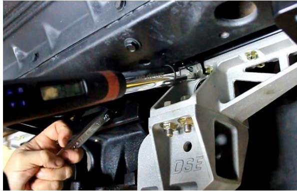
Figure 90 – Torque Upper Differential Bracket
