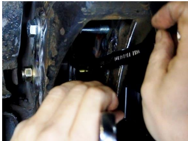
Figure 23 – Expand Crush Sleeve
