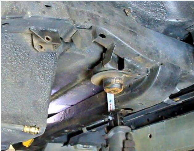
Figure 2 – Remove Frame Crossmember Brackets
