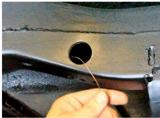
Figure 57 – Locate Lower Cradle Nut Plate
