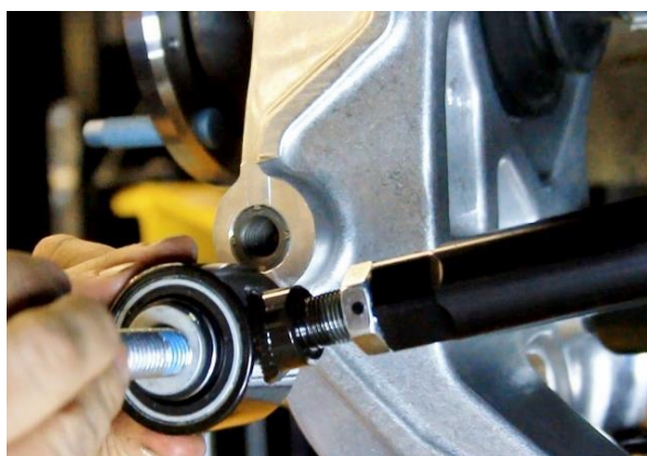
Figure 104 – Install Toe Links
