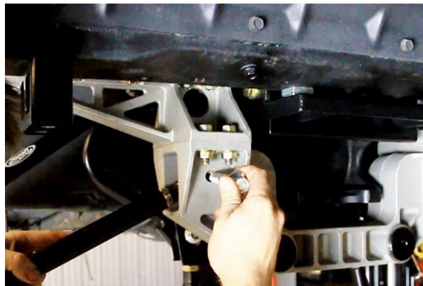
Figure 97 – Install Toe Link Assemblies
