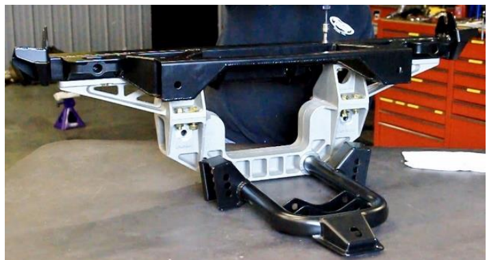
Figure 38 – Assemble the IRS Cradle
