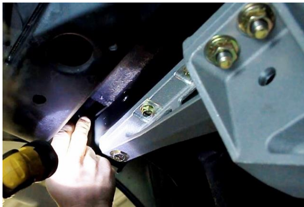
Figure 48 – Scribe Inside Mounting Hole Location
