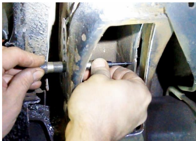
Figure 16 - Center Drill Inner Frame Rail
