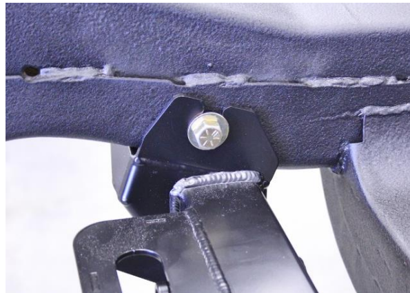
Figure 79 - Install Upper Cradle Assembly to Frame
