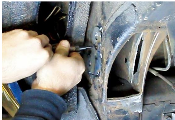
Figure 12 – Center Punch Trailing Link Holes
