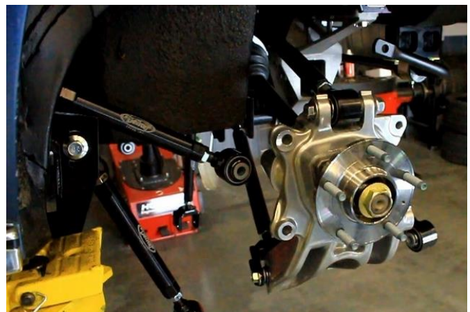
Figure 102 – Attach Lateral Links to Upright
