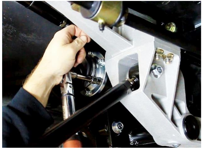
Figure 100 – Install Inner CV Joint to Stub Axle
