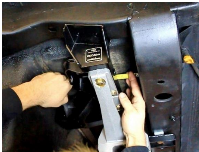
Figure 40 – Level IRS Cradle to the Frame
