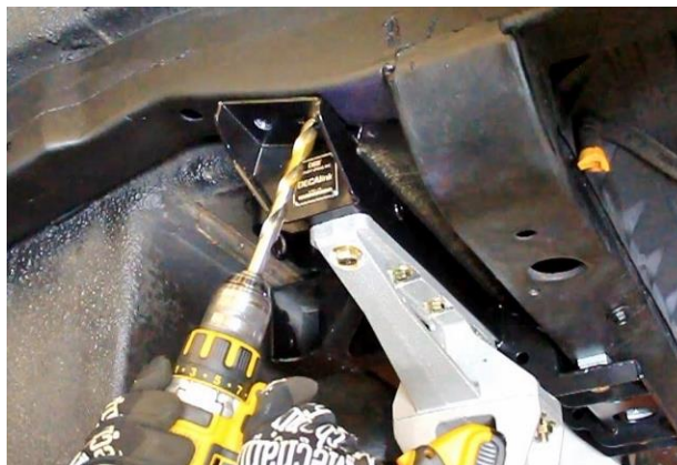
Figure 49 – Drill Bottom Side of Frame
