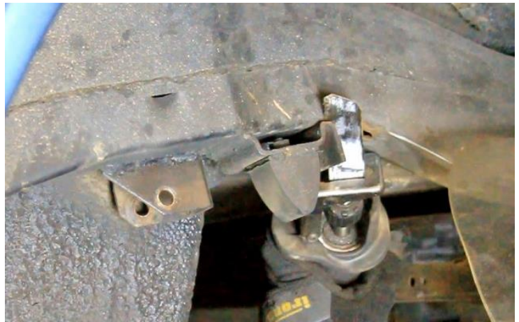
Figure 3 – Remove Frame Bumper and Upper Shock Mount Brackets
