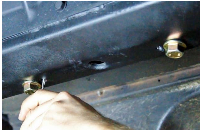
Figure 36 – Straighten Nut Plate & Clean Threads
