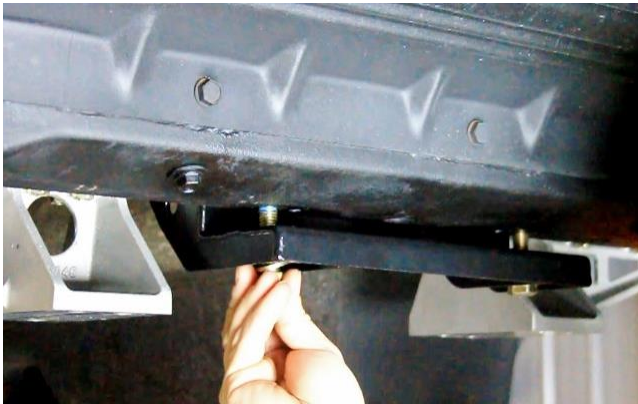
Figure 82 - Install Fasteners & Slotted Shims
