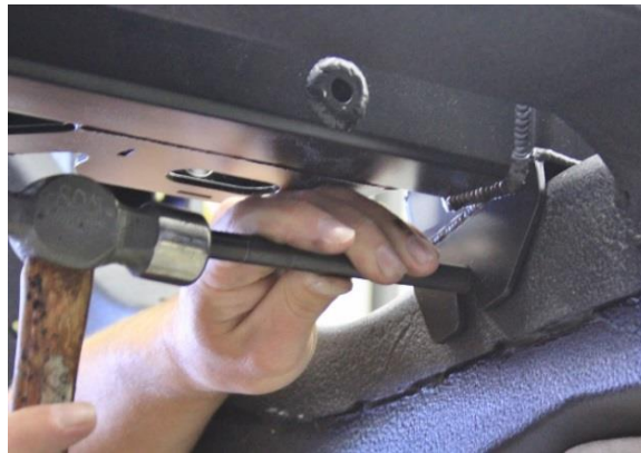
Figure 42 – Transfer Punch Frame for IRS Cradle
