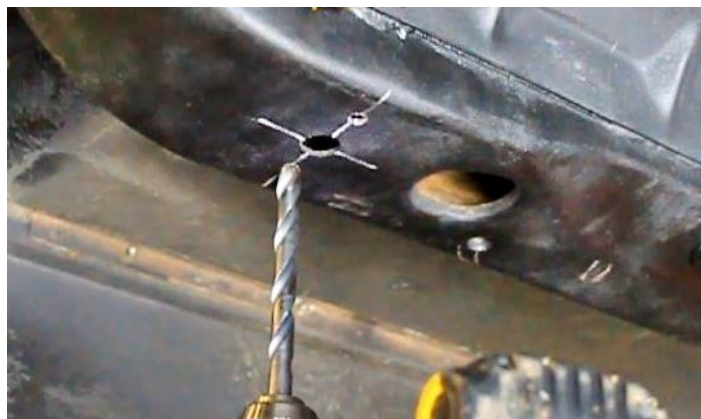
Figure 61 – Drill Sway Bar Nut Plate Location
