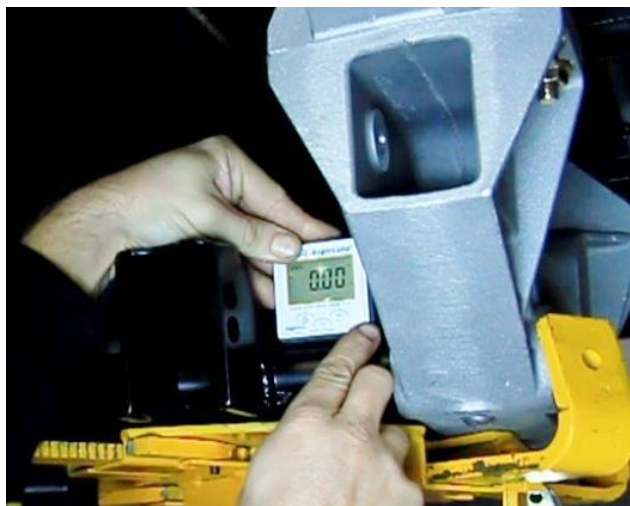
Figure 40 – Level IRS Cradle to the Frame
