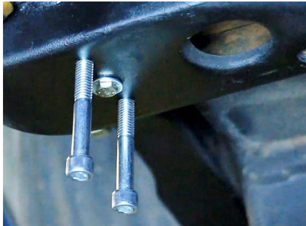
Figure 63 – Install Sway Bracket Nut Plate Assembly
