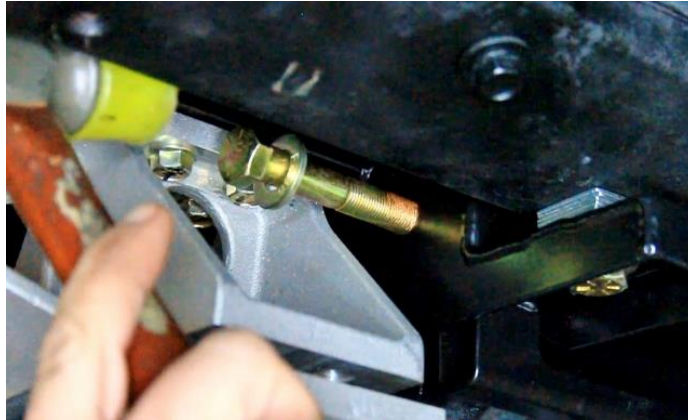
Figure 87 - Install Differential to Upper Cradle
