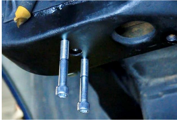
Figure 62 – Locate Sway Bar Nut Plate
