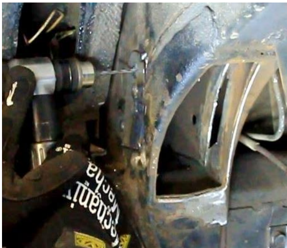
Figure 13 – Drill Trailing Link Holes
