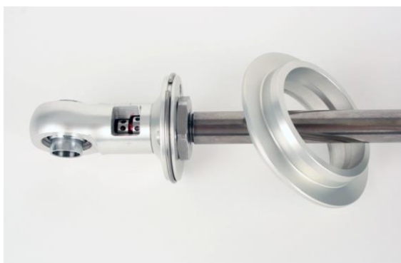
Figure 109 – Removing the Spring Seat
