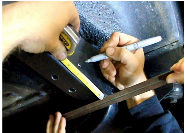
Figure 51 – Locate Access Holes
