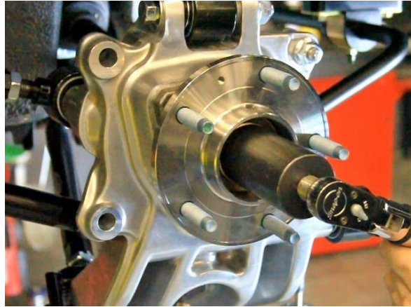
Figure 113 – Torque Outer CV Joint
