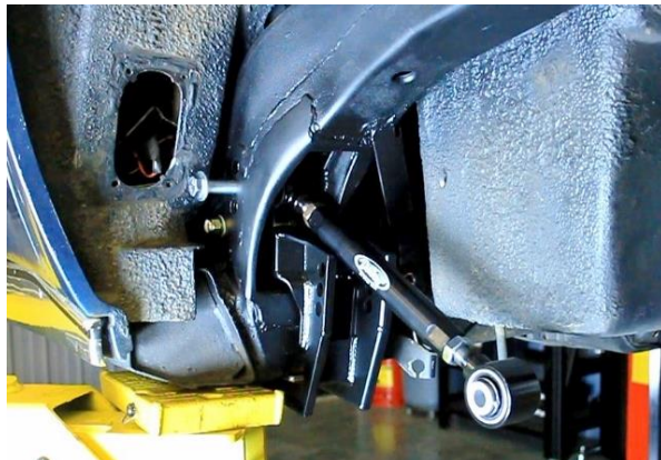
Figure 92 – Install the IRS Lower Trailing Links
