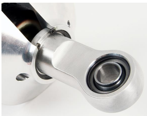
Figure 108 – Snap Ring Installed
