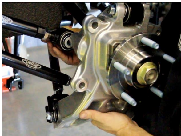
Figure 103 – Install Upper & Lower Trailing Links
