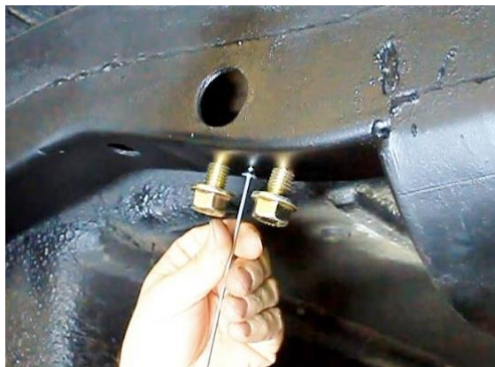
Figure 58 – Install Nut Plate Assemblies
