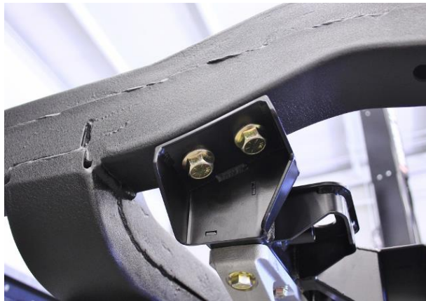
Figure 78 - Install Upper Cradle Assembly to Frame
