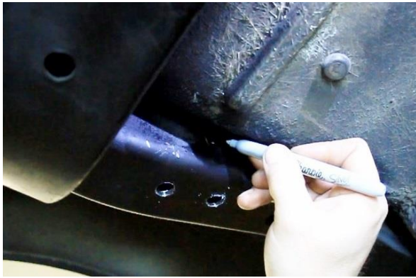
Figure 50 – Locate Inside Mounting Holes
