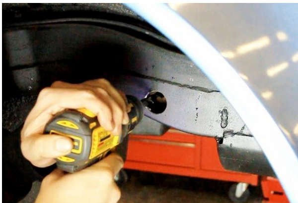
Figure 54 – Drill Inner Mounting Hole
