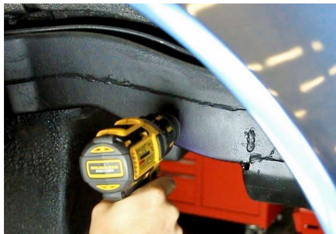
Figure 52 – Drill through Frame Rail
