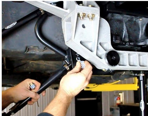
Figure 96 – Install Lower Lateral Links
