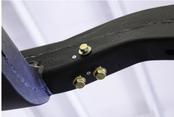
Figure 47 – Install Nut Plate Assemblies
