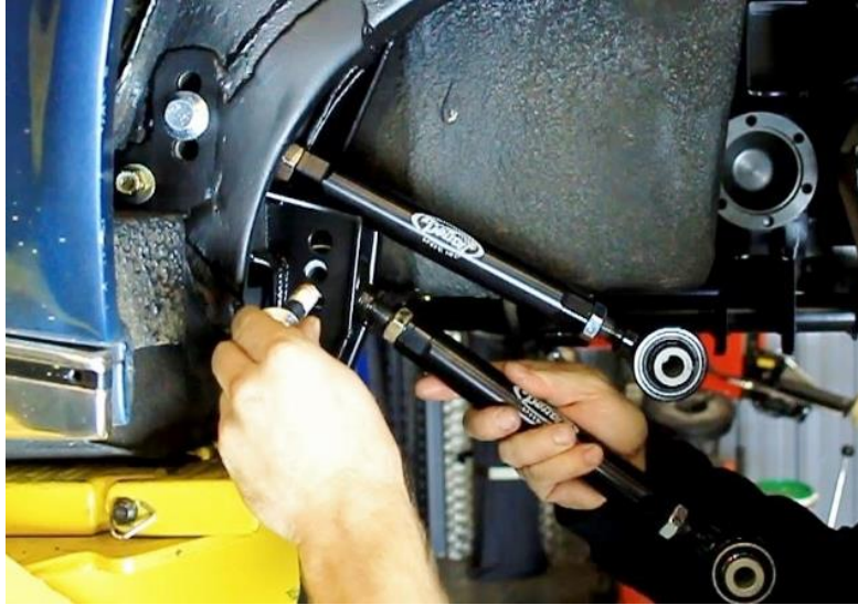
Figure 93 – Install the IRS Lower Trailing Links
