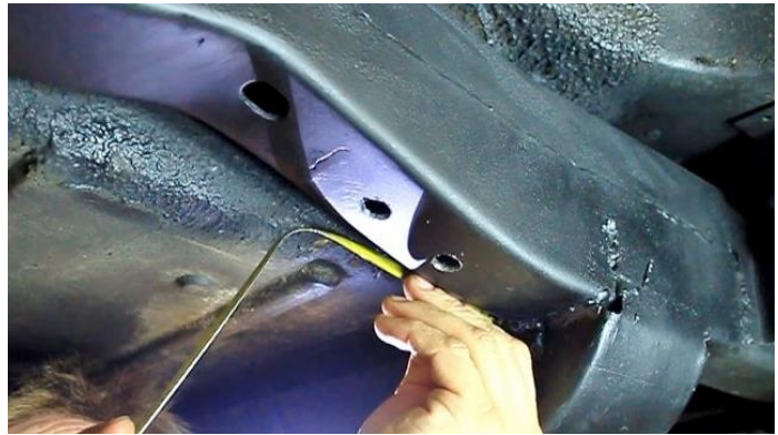
Figure 50 – Locate Inside Mounting Holes
