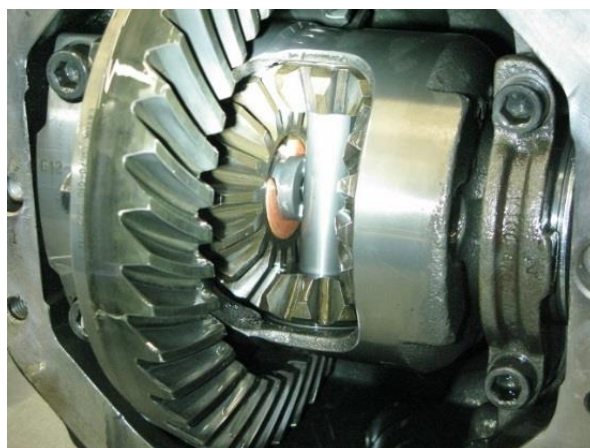
Figure 66 - Remove the Rear Cover
