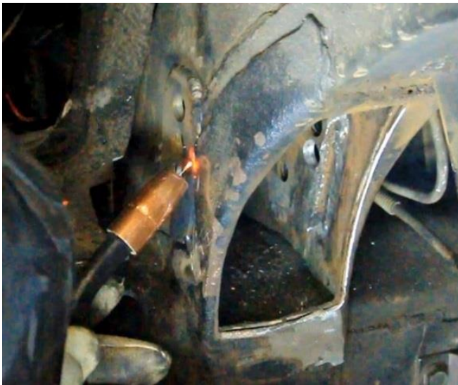
Figure 21 – Finish Weld Doubler Plates
