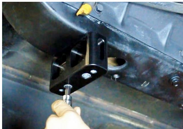
Figure 64 – Install Sway Bracket Spacer
