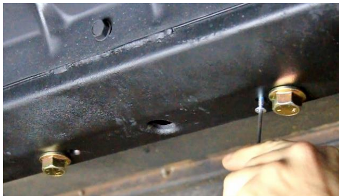
Figure 37 – Install Crossmember Nut Plate
