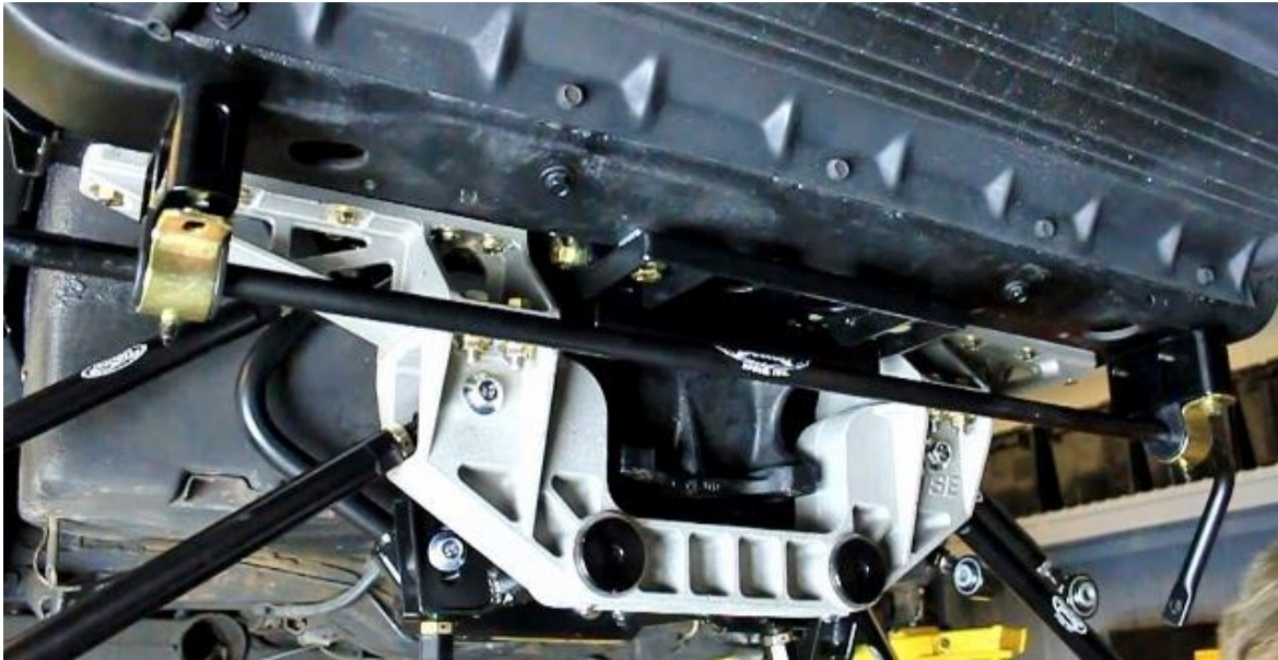
Figure 98 – Install Sway Bar
