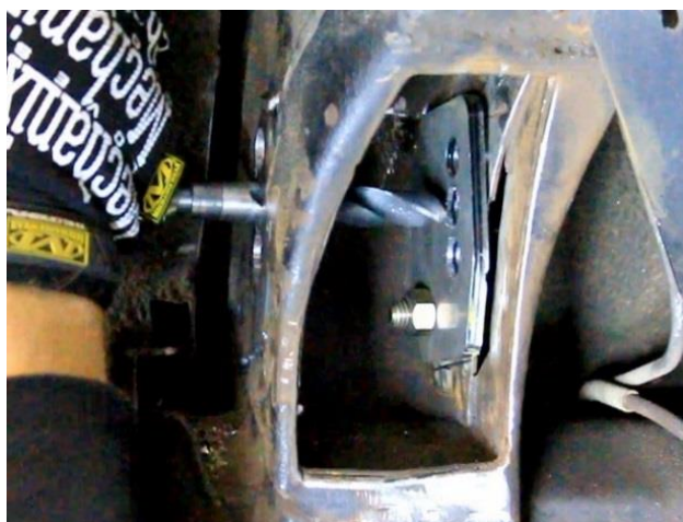
Figure 16 - Center Drill Inner Frame Rail
