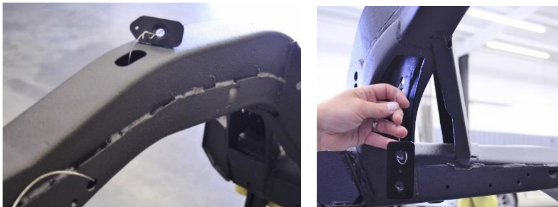
Figure 46 – Position Nut Plate Assemblies
