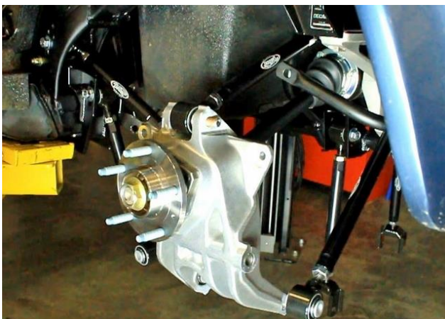
Figure 102 – Attach Lateral Links to Upright
