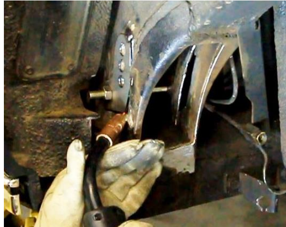
Figure 11 – Tack Weld Doubler Plate
