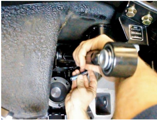
Figure 95 – Install Upper Lateral Link & Tie Braces
