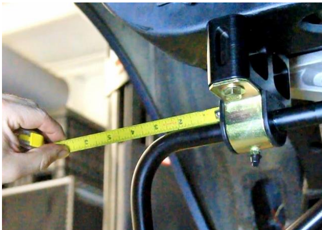
Figure 99 – Center Sway Bar and Install Split Lock Collars
