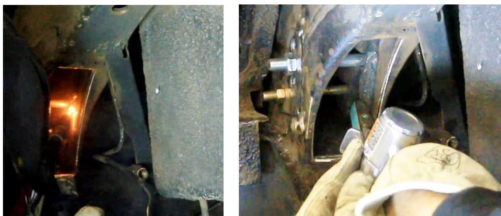
Figure 19 – Weld Inner Frame Rail
