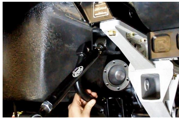
Figure 95 – Install Upper Lateral Link & Tie Braces
