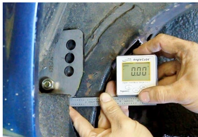
Figure 7 – Level Frame Doubler Plates
