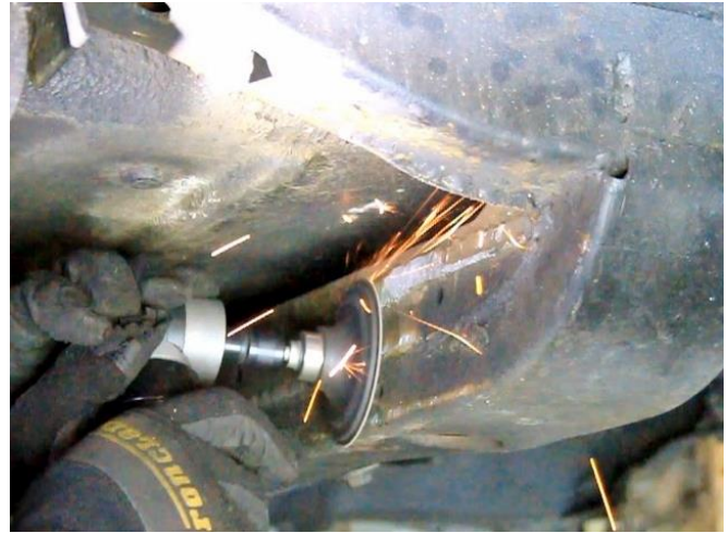
Figure 2 – Remove Frame Crossmember Brackets
