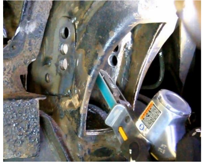
Figure 20 – Drill Upper & Lower Link Holes
