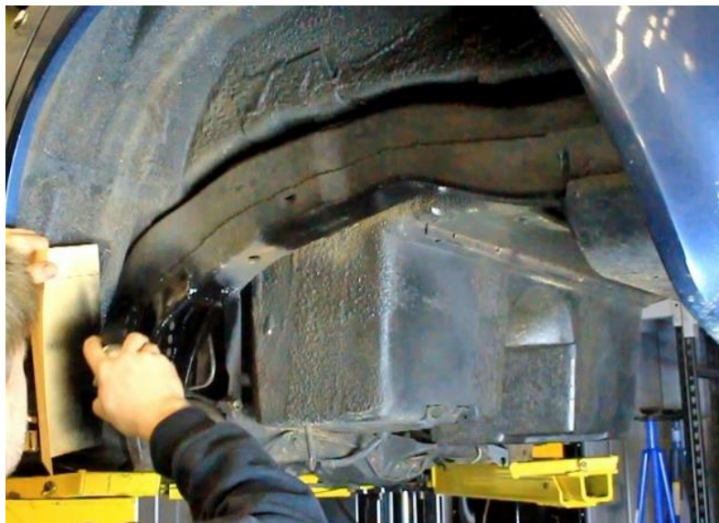
Figure 29 – Paint Modified Frame Rails
