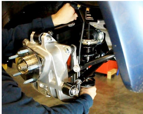
Figure 111 – Install Upper Shock Bolt & Spacer
