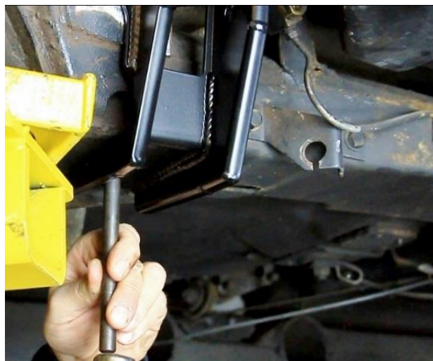
Figure 24 – Transfer Punch & Drill the Frame
