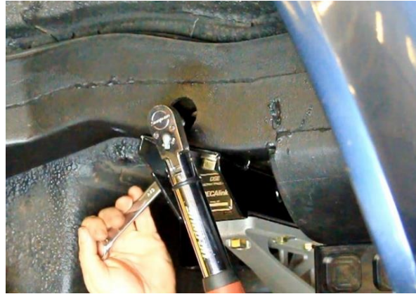
Figure 84 – Torque Inner Frame Rail Fasteners
