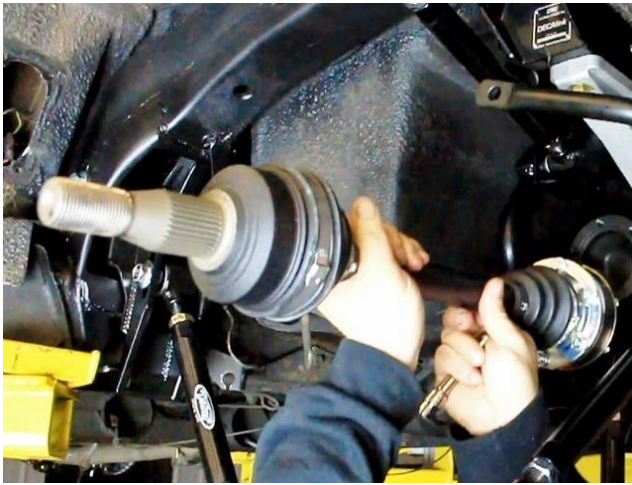
Figure 100 – Install Inner CV Joint to Stub Axle
