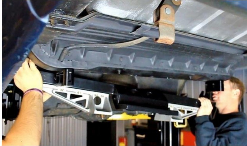
Figure 81 - Install Upper Cradle Assembly to Frame
