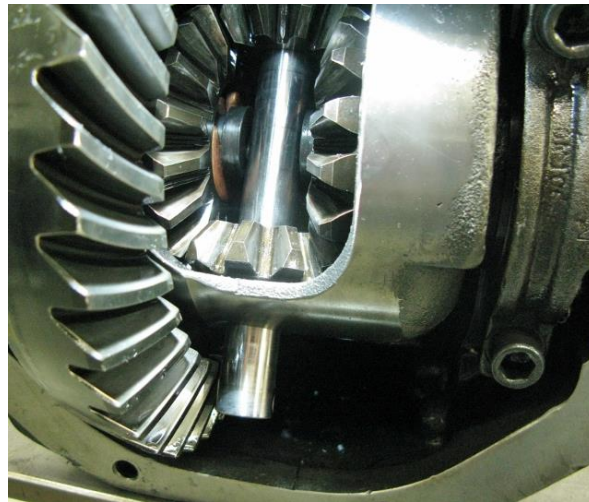
Figure 73 – Install Cross Shaft
