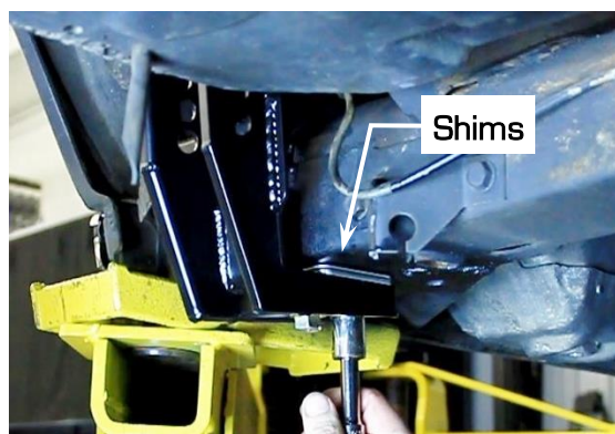
Figure 32 – Install Trailing Arm Bracket Assembly
