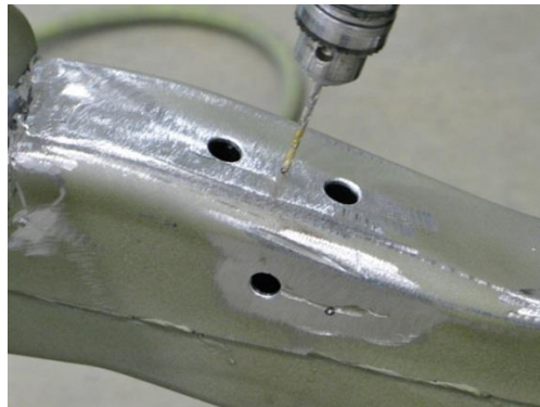
Figure 45 – Drill & Chamfer Nut Plate Locators
