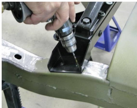
Figure 43 – Drill IRS Cradle Mount Locations
