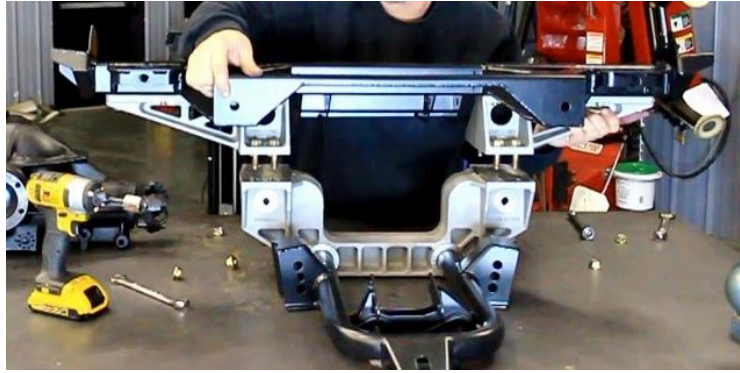
Figure 75 – Disassemble IRS Upper & Lower Cradle
