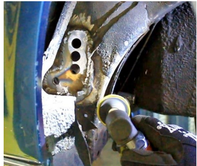
Figure 21 – Finish Weld Doubler Plates
