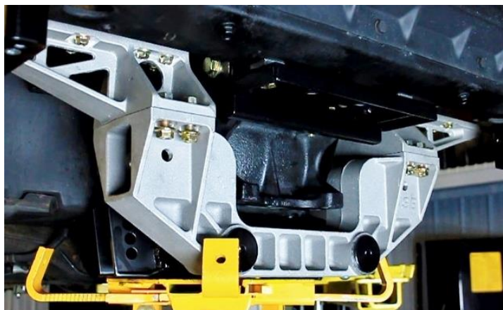
Figure 89 - Assemble the IRS Upper and Lower Cradle
