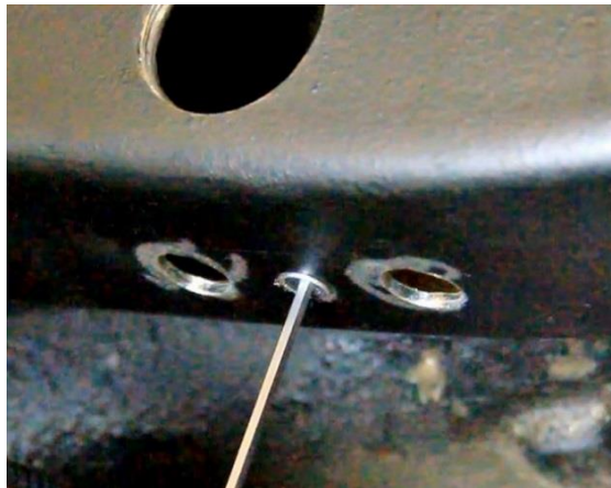
Figure 56 – Drill & Chamfer Nut Plate Locators
