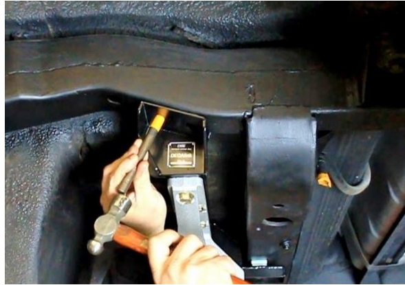
Figure 41 – Transfer Punch Frame for IRS Cradle
