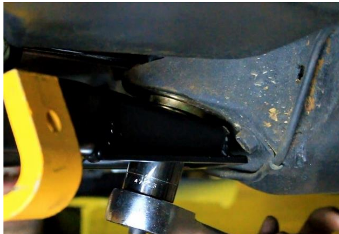
Figure 88 - Torque Lower Differential Mount
