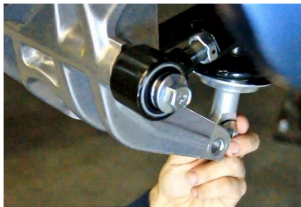
Figure 112 – Install Lower Shock Bolt & Tapered Spacers
