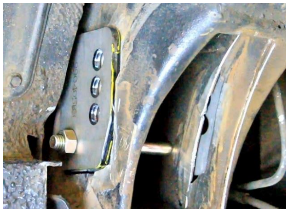
Figure 10 – Verify Frame Rail Modification
