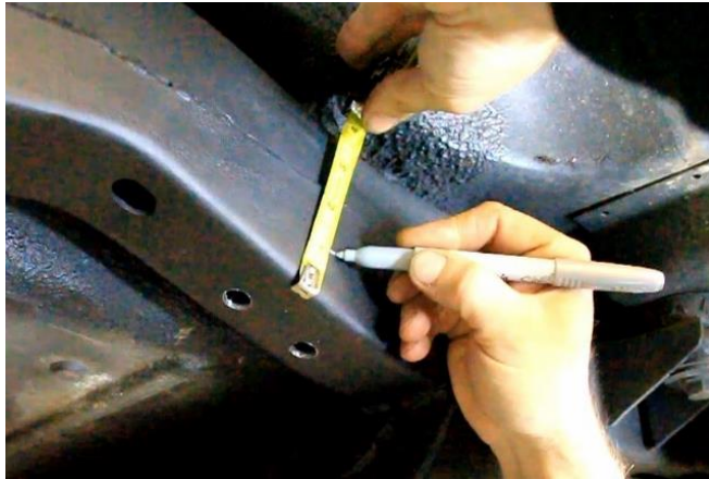
Figure 51 – Locate Access Holes
