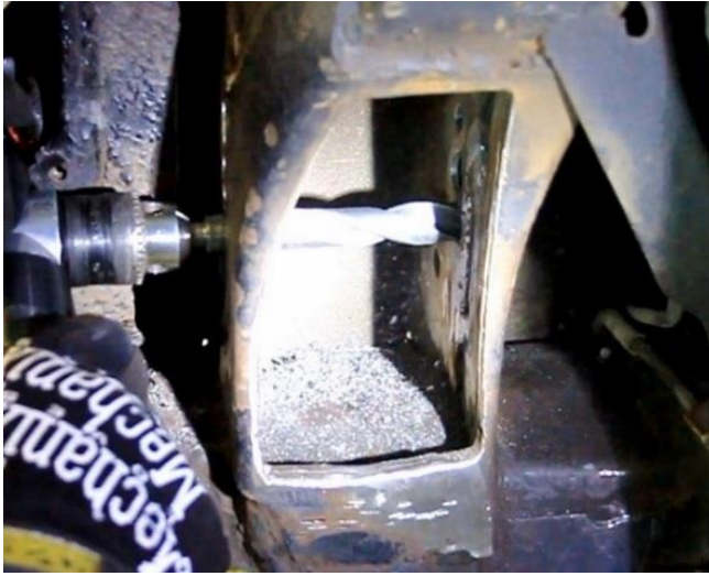
Figure 20 – Drill Upper & Lower Link Holes
