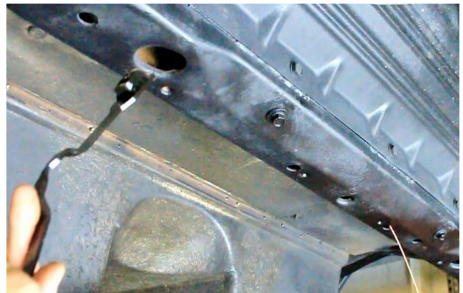
Figure 35 – Bend Crossmember Nut Plate
