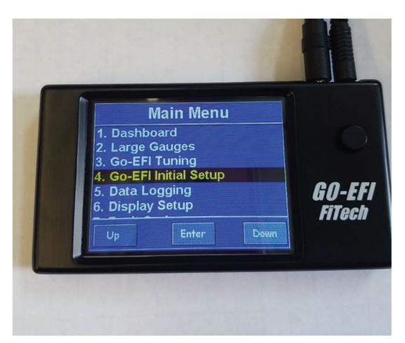
**Step 3:** go under option 1: engine setup. Then, scroll down to option 6 (pump PWM/FCC) and select edit, press clear (CLR) and enter a new value. The lower the number the slower the pump will run. **If you have a "Tank's Inc." #2 or #4 series pump set the value to 100.** Press ok, then in the fuel pump control menu press the center of the control stick to send the change to the ECU.
