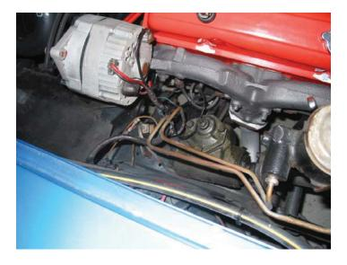
2. Once, drained, remove original non-power Master Cylinder and Master Cylinder lines.
