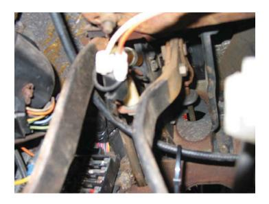
7. Remove the push rod from the pedal and the stop light switch bracket, these will be replaced.
