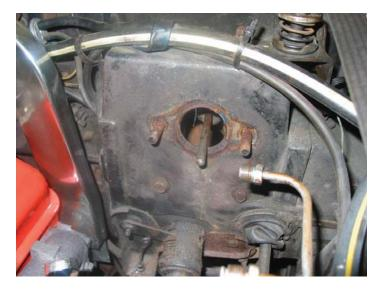
3. Once the Master Cylinder is removed, you will need to remove the upper studs by driving them out with a hammer and the lower bolts on the firewall. These two bolts help hold the pedal assembly to the firewall, the new brake booster will have studs that will replace these.
