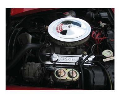
10. You can now install the power master cylinder. Once it is mounted you can install the new power master cylinder lines.
