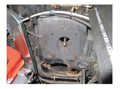
4. Using the supplied brake booster gasket, align it with the lower holes on the firewall. Using a silver marker draw the center hole and the four bolt holes for the booster. The bottom holes are in the correct position but will need to be opened up.
