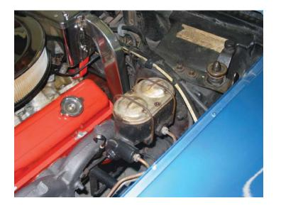
1. Remove the brake fluid from the Master Cylinder, usually a cheap turkey baster will work well for this. Please note that brake fluid is caustic so it will damage your paint if you get any on it.
