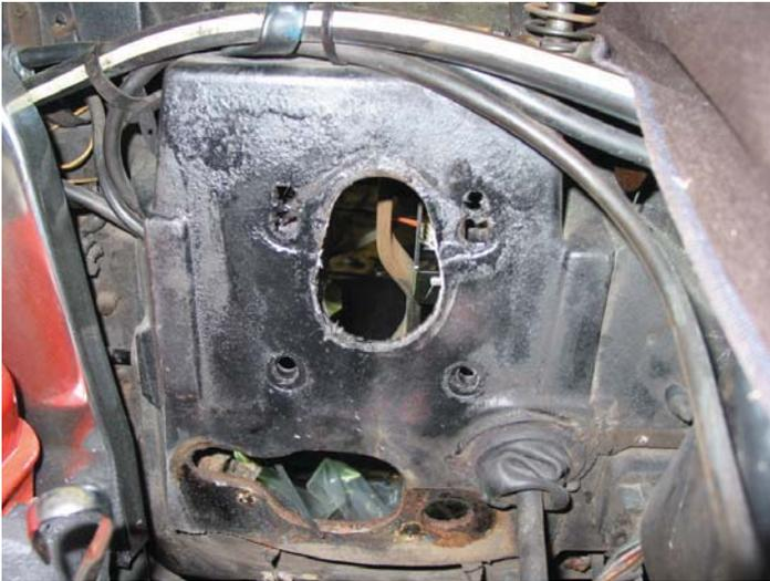
5. Drill a small pilot hole through the top hole, once you have done this follow through with a 3/8 drill on both the top and bottom holes.
