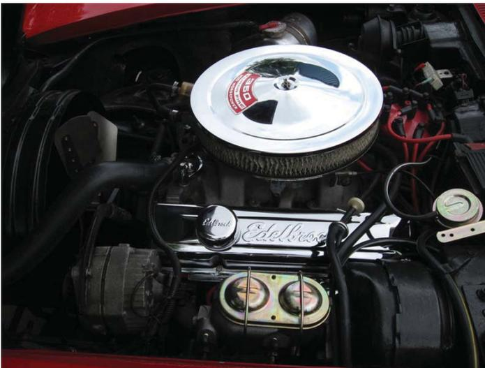
10. You can now install the power master cylinder. Once it is mounted you can install the new power master cylinder lines.
