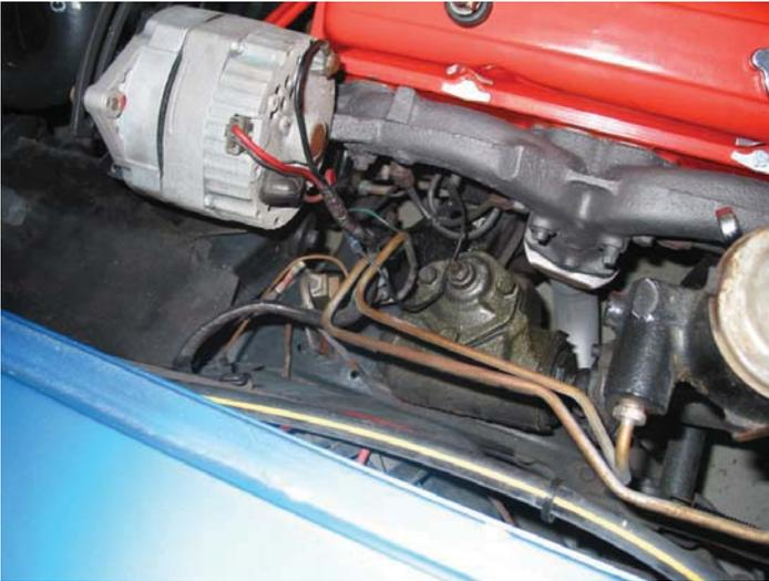
2. Once, drained, remove original non-power Master Cylinder and Master Cylinder lines.
