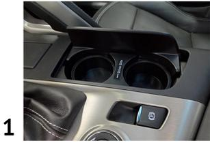
**PHOTO 1 – THE STOP FLOP CUP HOLDER MOUNTS INTO THE FACTORY CONSOLE TRAY WITH SUPPLIED SELF-ADHESIVE TAPE.**
