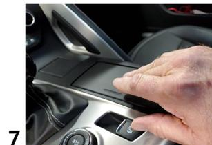
**PHOTO 6 & 7 – CUP HOLDER REINSERTED INTO CONSOLE AND LID CLOSURE.**
