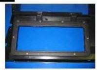
Guide radiator shroud into place, using caution not to damage the A/C condenser.
