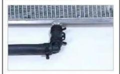
Fill the intercooler coolant system with coolant removed in previous step.
