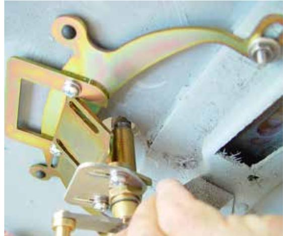
(Fig 9-4) Insert the Pivot Shaft with the Pivot Shaft Orientation Bracket upward toward the corresponding wiper shaft hole in the fiberglass cowl. This car does not have the metal substructure but illustrates how the Pivot Shaft is re-installed after the Pivot Shaft Mounting Plate has been installed.
