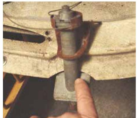
(Fig 2-4) Remove the pivot shafts.
