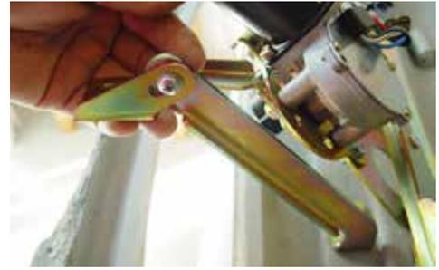
(Fig 13-2) Attach the other end of the to the Windshield Brace to the Windshield Brace Mounting Bracket mounted under the Cover Plate.
