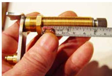
(Fig 3-8) Run a 5/8-24 hex nut down the threads of each pivot shaft about 2 3/8"
