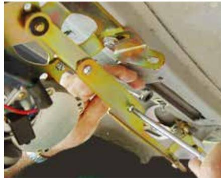
(Fig 11-3) Passenger side Link length adjustment. Loosen the two phillips head screws that attach the long and short Link halves. Slide them apart or together to adjust the length.
