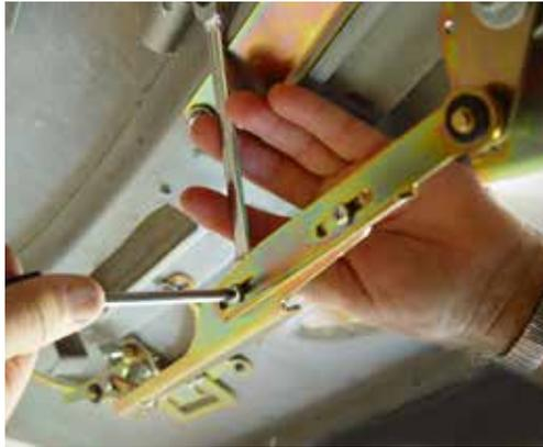
(Fig 12-1) Driver side Link length adjustment.
