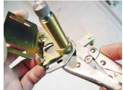
(Fig 4-3) It doesn't go on the shaft easily. You might find it easier to gently hold the Pivot Shaft with vice grips.
