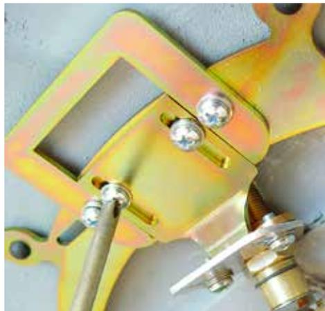
(Fig 9-5) A primary adjustment is by loosening the four phillips head screws in the Pivot Shaft Orientation Bracket. The inside two give front to back (in and out) adjustment. The outside two give side to side adjustment.
