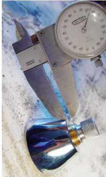
(Fig 10-1) With the chrome escutcheon placed onto the Pivot Shaft and resting on the body, 1/8" to 3/16" of the brass threads of the Pivot Shaft should be showing.
