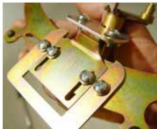
(Fig 4-6 & 4-7) Using the 10-32x3/8" phillips head screws and washers, attach the Pivot Shaft Orientation Bracket to the Pivot Shaft Mounting Plate.
