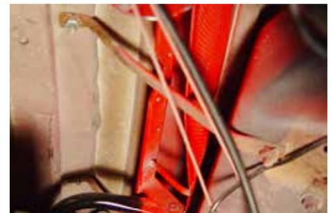
(Fig 2-6) Remove the right, or passenger side windshield brace rod.
