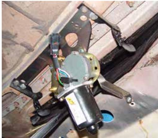
(Fig 7-5) Place the Main Drive Unit up against the underside of the cowl, between the cowl vent hinge brackets. Use four 1/4-20x3/8" hex bolts and 1/4" flat washers to hold the Main Drive Unit and cowl vent brackets in place.
