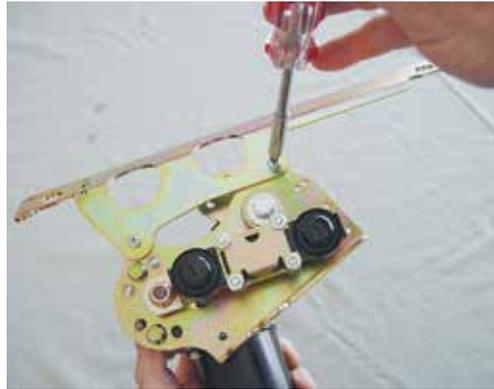
(Fig 7-1) Using two 10-32x3/8 screws, nuts and washers, attach the motor to the motor mount bracket.
