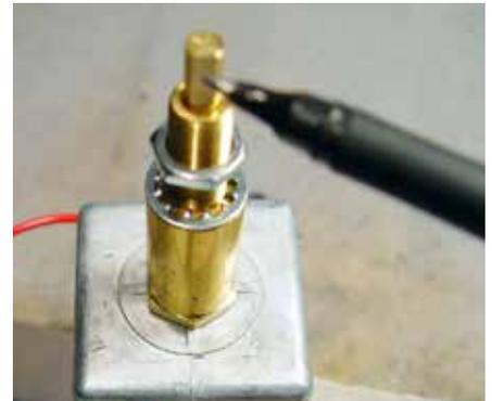
(Fig 13-4) File enough to allow the set screw to securely clamp the knob to the shaft.
