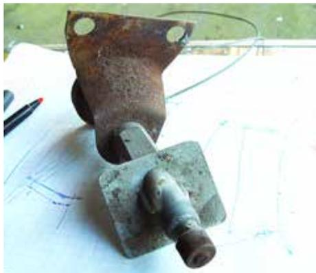
(Fig 2-5) The pivot shaft after being removed.
