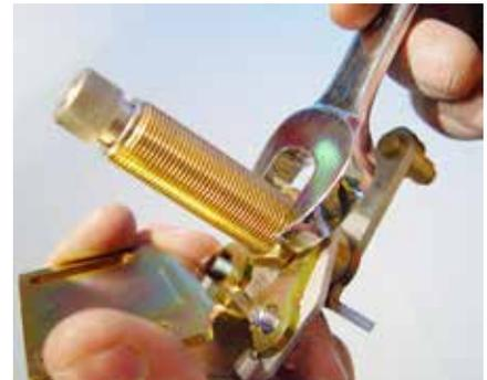
(Fig 4-5) Run the hex nut down to the Pivot Shaft Orientation Bracket about finger tight.
