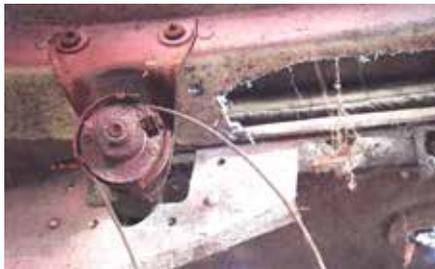
(Fig 2-3) On 1956-57, remove the spool and cable assembly.
