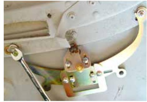
(Fig 9-2) Place #12-24 hex nuts and 1/4" flat washers on the windshield retaining studs and tighten them.
