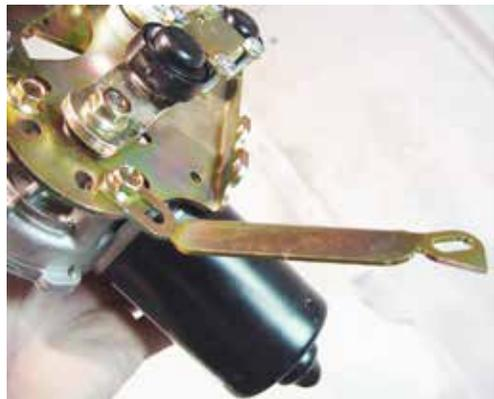
(Fig 7-3) Attach the Motor Brace.
