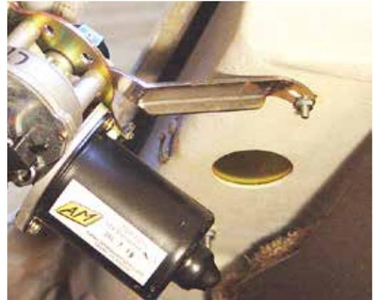
(Fig 12-4) The Motor Brace was attached to the cowl so the wiper unit could be installed and adjusted. The Windshield Brace Mounting Bracket will be added at that location.
