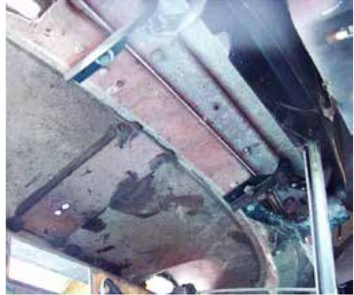
(Fig 7-4) Remove 4 1/4-20 hex bolts holding the cowl vent hinge brackets to the under side of the cowl.
