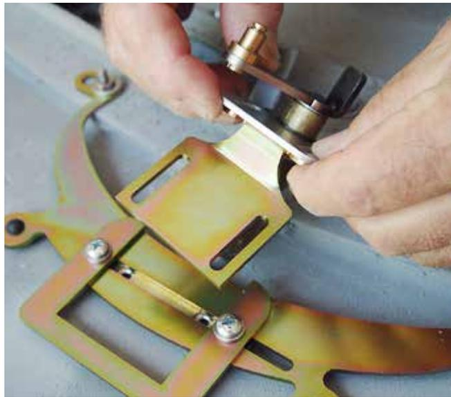
(Fig 8-2) If your Corvette has a metal substructure, side to side, under the windshield, you will need to remove the Pivot Shaft Orientation Brackets from the Pivot Shaft Mounting Plates. If it does not, this step is optional.
