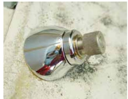
(Fig 10-5 & 10-6) When you are satisfied with the fit of the Pivot Shaft and chrome escutcheon fit on the outside of the car, tighten all interior screws before installing the chrome escutcheon nut with the aluminum Escutcheon Wrench supplied in the kit. Overtightening can damage the fiberglass.
