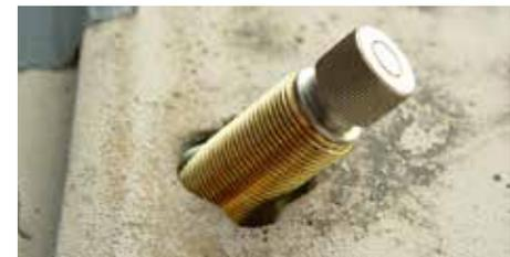
(Fig 9-6) The Pivot Shaft should be centered within the hole in the cowl.
