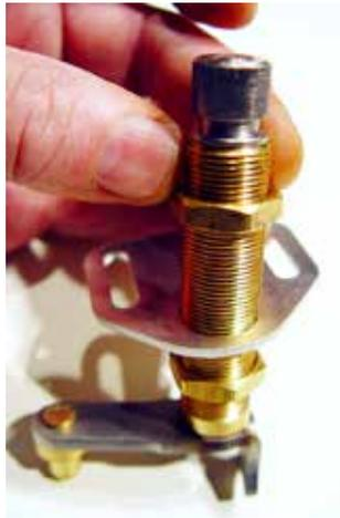
(Fig 4-1) Add the flat aluminum Pivot Shaft Holding Plate down to the first hex nut and install a second 5/8-24 hex nut.
