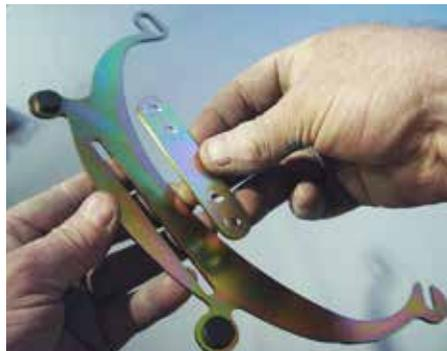
(Fig 3-6 & 3-7) On the opposite side of the pivot shaft Mounting Plate, the 4 nut backing strip is used to attach the "U" Guide to the Mounting Plate.
