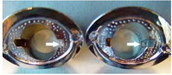
(Fig 3-2) Each early chrome escutcheon is marked "R" or "L" on the backside down inside the slots.
