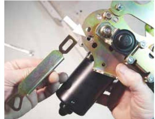
(Fig 7-2) Use a 10mm wrench to remove the motor mounting screw as shown
