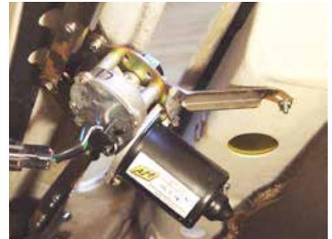
(Fig 7-6) The opposite end of the Motor Brace goes up against the underside of the firewall where the left side of the old (OEM) wiper motor was attached. Attach the Brace using a 10-32x3/4" phillips, washer, and nut. This same fastener holds one side of the new Cover Plate.
