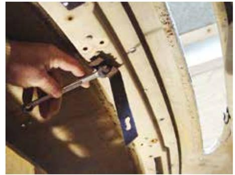
(Fig 2-2) Remove the radio support.
