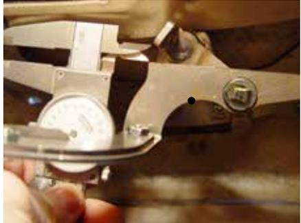
(Fig 11-4) When the Pivot Shaft is in the parked position, there should be between a 1/4" to 3/16" gap between the flat in the Cross Link end and the stop tab on the Pivot Shaft.
