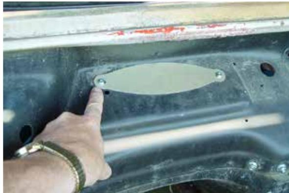
(Fig 12-5) The Cover Plate goes where the old motor was mounted.
