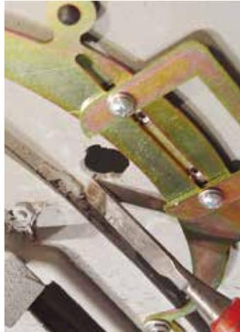
(Fig 9-3) Some Corvettes need the excess glue, aft of the pivot shaft, removed so the new pivot shaft will fit properly.
