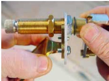
(Fig 10-3) Loosen the 5/8-24 hex nut closest to the tip and rotate it toward the tip by the distance you want to pull the tip closer to the cowl.
