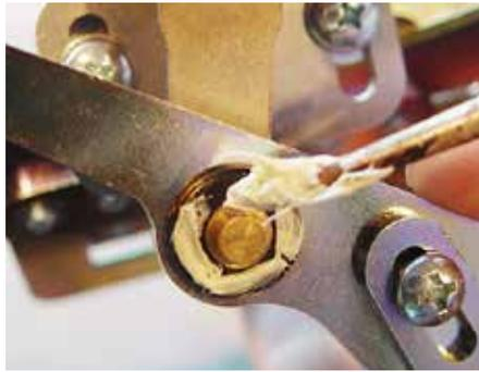
(Fig 11-01) Put a dab of thick axle grease on the exposed side of the plastic bushing before placing the very thin flat washer onto the exposed brass pivot pin, sticking it to the grease on the plastic bushing.
