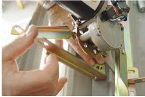
(Fig 13-1) Attach the Windshield Brace on the middle right hand windshield attachment bolts.
