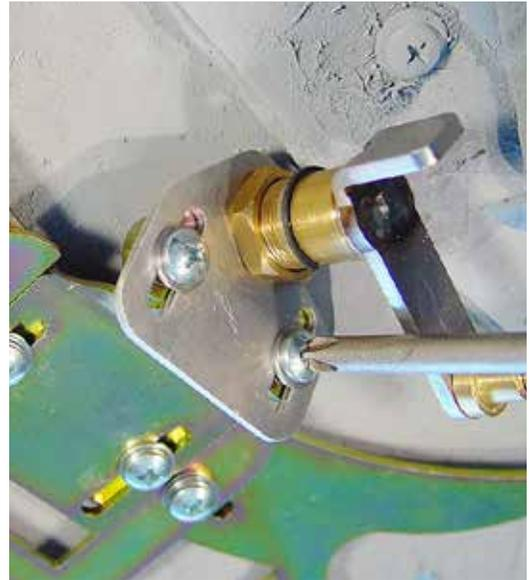
(Fig 10-2) The other primary, up and down, adjustment is by loosening the two phillips head screws of the aluminum Pivot Shaft Holding Plate so it can be adjusted.
