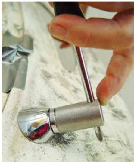
4f. To seal the pivot shaft hole in the cowl, place body sealer on the bottom of the escutcheon before final installation.
