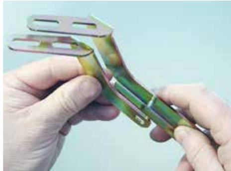
(Fig 5-4) Match the outer end of the longer Link to the Link End Stiffener.
