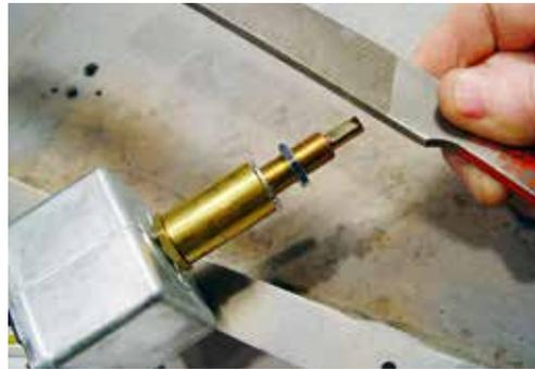
(fig 13-3) File a flat spot in the shaft at the 6 o'clock position for the switch knob's set screw.
