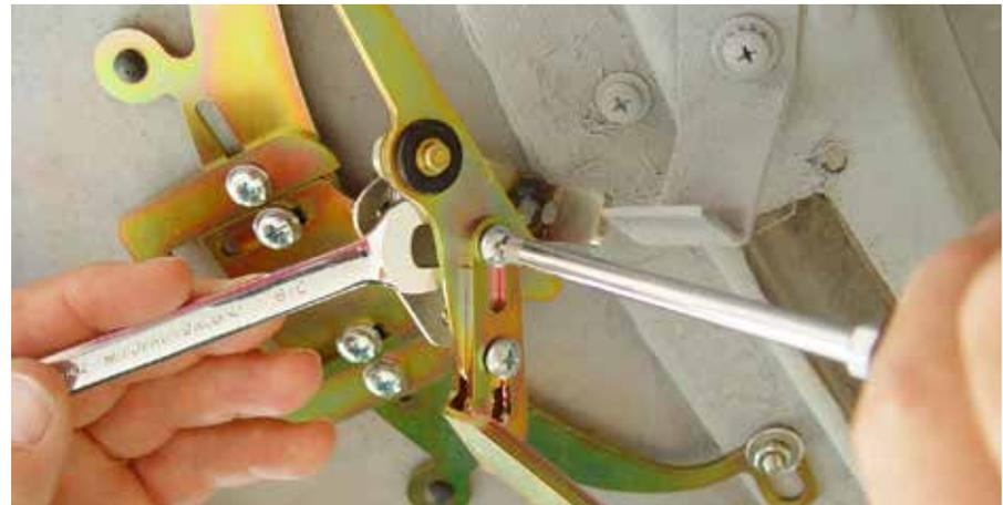
(Fig 11-5) On the driver side loosen the two phillips head screws, extend or retract the Link Tip as needed clear both the defroster duct and the brake pedal/clutch pedal bracket. Retighten the screws.
