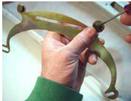
(Fig 3-4) Using a small tip screwdriver, install 2 rubber bumpers in each part so that the bumpers for each part is on the top side.
