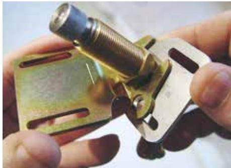
(Fig 4-2) Slip the tips of the open end of the Pivot Shaft Orientation Bracket onto the brass Pivot Shaft.
