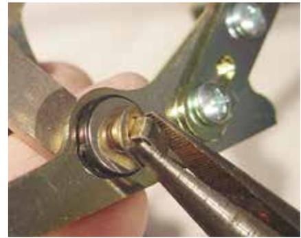
(Fig 11-02) Grab a spring clip with a pair of needle nose pliers. Slip the spring clip over the brass pivot pin, press towards the thin washer/plastic bushing and secure the clip into the groove in the shaft.
