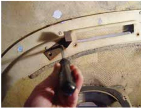
(Fig 2-1) On 53-55 Corvettes you do not need to remove the stock pivot shaft brackets. On 1956-57 Corvettes you do.
