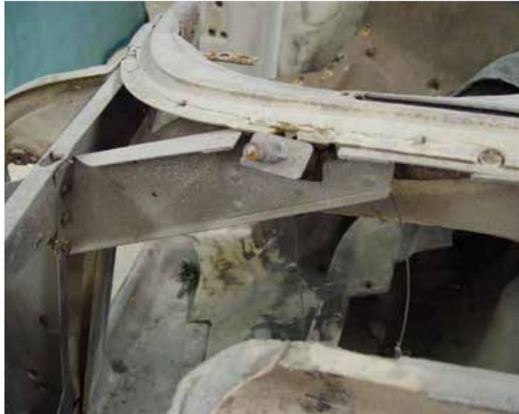
(Fig 8-1) This is the passenger side looking aft. The fiberglass cowl has been removed. This Corvette has the metal substructure that requires separating the Pivot Shaft Orientation Brackets from the Pivot Shaft Mounting Plates and "U" Guides to install the Pivot Shaft Mounting Plates and "U" Guides between the metal substructure and fiberglass cowl.
