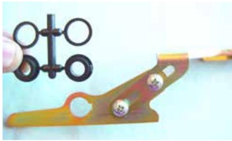
(Fig 6-1) The Plastic Bushings that fit into the keyed holes in the Link Tips & opposite Link ends.
