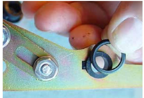
(Fig 6-5) The Plastic Bushings that fit into the keyed holes in the Link Tips have a plastic ring that fits on the side that extends through the keyed hole.
