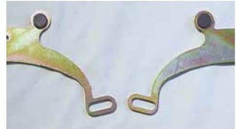
(Fig 3-5) The bumpers have been installed on the top of both brackets.
