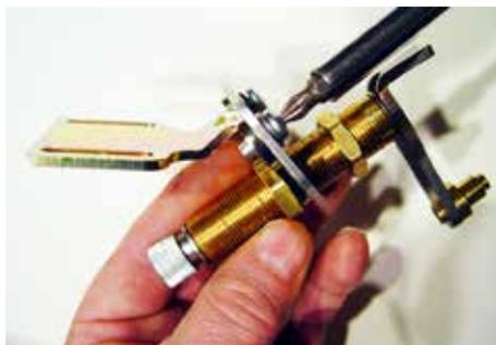
(Fig 4-4) Using two 10-32x3/8" phillips head screws and flat washers, attach the aluminum Pivot Shaft Holding Plate to the Pivot Shaft Orientation Bracket.
