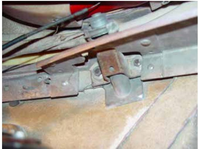
(Fig 02-02) Remove the spool and cable assembly.
