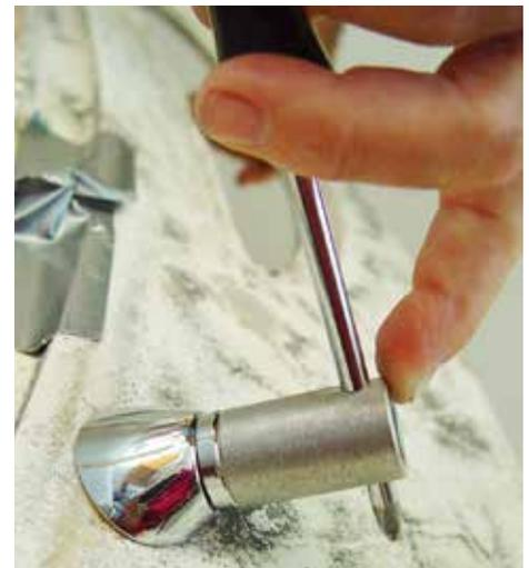
(Fig 06-06) When you are satisfied with the fit of the Pivot Shaft and chrome escutcheon fit on the outside of the car, tighten all interior screws before installing the chrome escutcheon nut with the aluminum Escutcheon Wrench supplied in the kit. Overtightening can damage the fiberglass.
