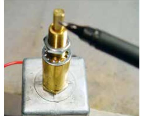
(Fig 09-04) File enough to allow the set screw to securely clamp the knob to the shaft.
