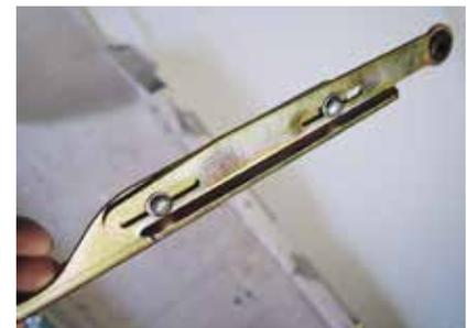
(Fig 03-07) Attach the short Link to the other end of the longer Link assembly.
