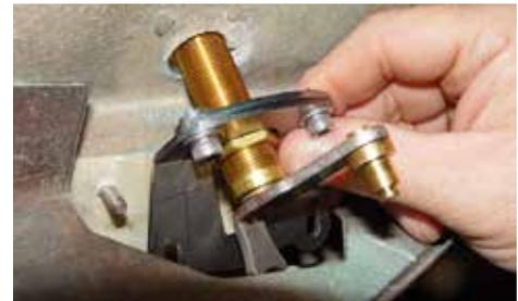
(Fig 06-02) Place the two shotted holes onto the 10-24 studs.
