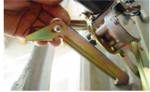
(Fig 09-02) Attach the other end of the Windshield Brace to the Windshield Brace Mounting Bracket mounted under the Cover Plate.
