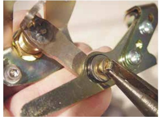
(Fig 07-02) Grab a spring clip with a pair of needle nose pliers. Slip the spring clip over the brass pivot pin, press towards the thin washer/plastic bushing and secure the clip into the groove in the shaft.
