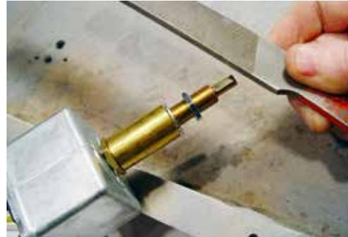
(Fig 09-03) File a flat spot in the shaft at the 6 o'clock position for the switch knob's set screw.
