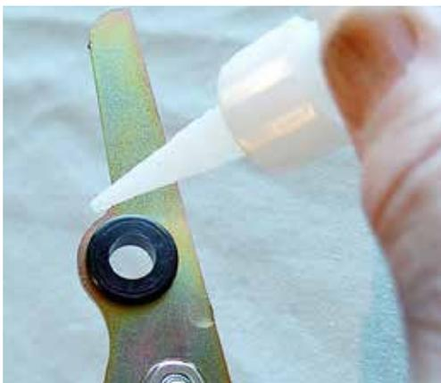
(Fig 04-06) Use a very thin bead of super glue to secure the Plastic Ring to the Plastic Bushing.
