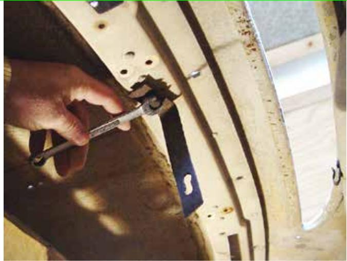
(Fig 02-01) Remove the radio support.
