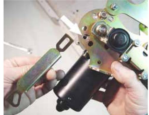
(Fig 05-02) Use a 10mm wrench to remove the motor mounting screw as shown
