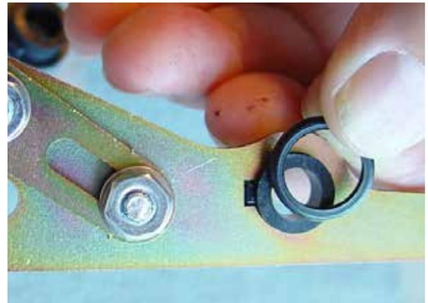
(Fig 04-05) The Plastic Bushings that fit into the keyed holes in the Link Tips have a plastic ring that fits on the side that extends through the keyed hole.
