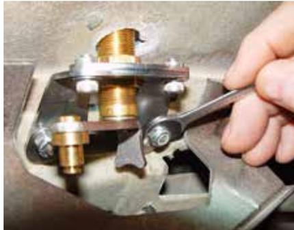
(Fig 06-03) Secure the Pivot Shaft Bracket to the body.
