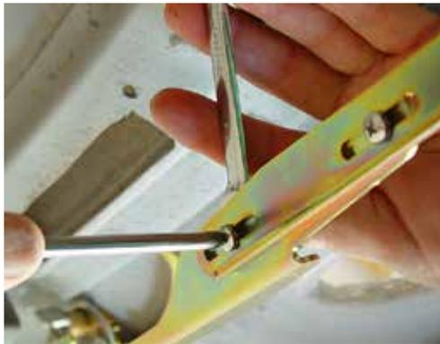
(Fig 08-01) Driver side Link length adjustment.
