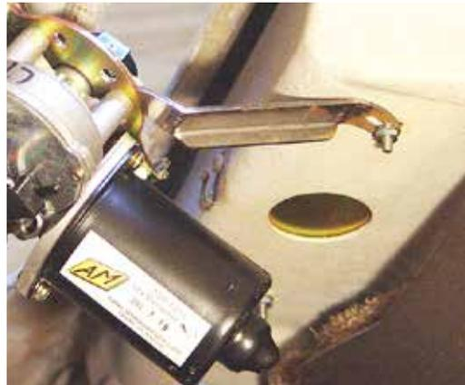
(Fig 08-04) The Motor Brace was attached to the cowl so the wiper unit could be installed and adjusted. The Windshield Brace Mounting Bracket will be added at that location. (53-57 shown)
