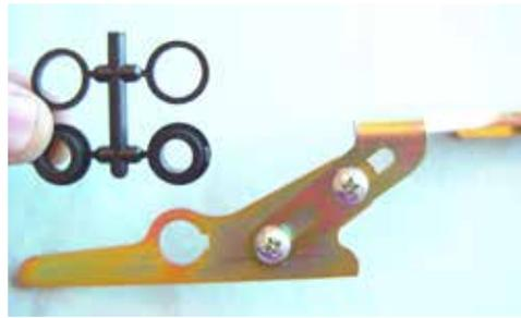
(Fig 04-01) The Plastic Bushings that fit into the keyed holes in the Link Tips & opposite Link ends.
