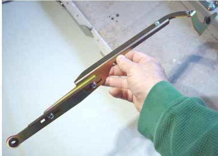
(Fig 03-03) The complete passenger side Link assembly with the longer and shorter links attached.
