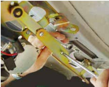
(Fig 07-03) Passenger side Link length adjustment. Loosen the two phillips head screws that attach the long and short Link halves. Slide them apart or together to adjust the length.
