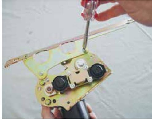
(Fig 05-01) Using two 10-32x3/8 screws, nuts and washers, attach the motor to the motor mount bracket.
