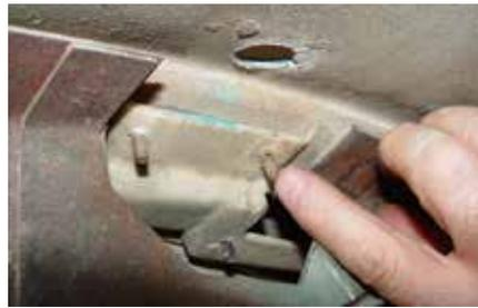
(Fig 06-01) Locate the original pivot shaft bracket studs.
