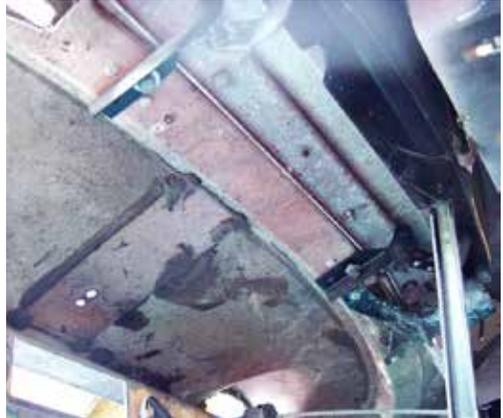
(Fig 05-04) Remove 4 1/4-20 hex bolts holding the cowl vent hinge brackets to the under side of the cowl.
