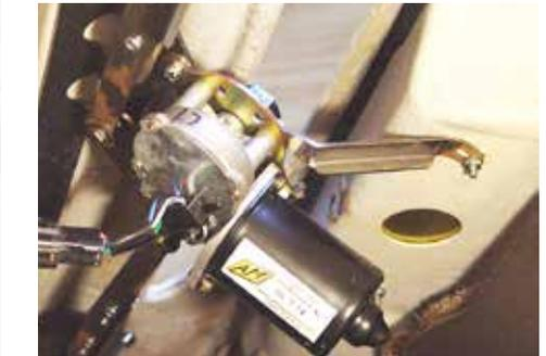
(Fig 05-06) The opposite end of the Motor Brace goes up against the underside of the firewall where the left side of the old (OEM) wiper motor was attached. Attach the Brace using a 10-32x3/4" phillips, washer, and nut. This same fastener holds one side of the new Cover Plate.
