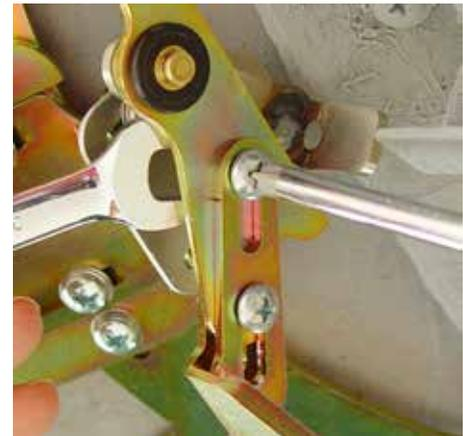
(Fig 07-05) On the driver side loosen the two phillips head screws, extend or retract the Link Tip as needed clear both the defroster duct and the brake pedal/clutch pedal bracket. Retighten the screws.
