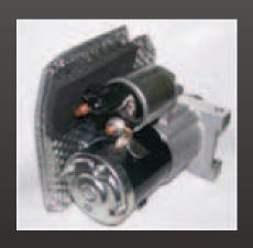
Before starting disconnect the battery to avoid electrical shorts during the installation of the shield.
