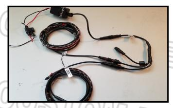
This image shows the 3 way splitter installed between the control box and the engine bay strips. The empty connector gets connected to the coil cover kit. Be sure to align the Arrows on the connectors when plugging them in. Test the strips before mounting them.
