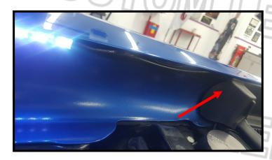
Mount the strip on the passenger side in the same fashion as the drivers side. You can start the strip near the black cover (red arrow) but the end wont line up with the strip on the other side. Alternatively you can mount it as shown and secure the wire with gorilla tape. Route the wire behind the black cover. The wire for the passenger side is extra long so you will have to hide the extra down inside the fender.
