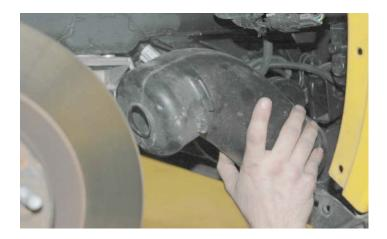
82. Unbolt the horn assembly with a 13mm wrench
