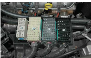
191. Gently remove the wire cover from the bottom of the DARK GREY wiring block by prying up on the clips that retain the cover on each end. This will expose the wire connections on the bottom of the block.
