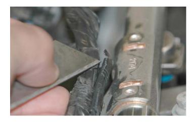
42. Disconnect the eight fuel injector connectors by pressing in on the release triggers and pulling the connectors free.
