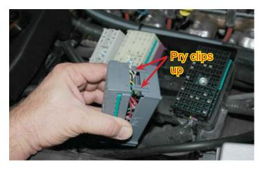
192. Here is the DARK GREY wiring block with the bottom cover removed showing the wiring. Note: The wire connections are lettered across the top and numbered down the side. Locate the GREY wire in the A7 location. This is the wire we will be making connections to.
