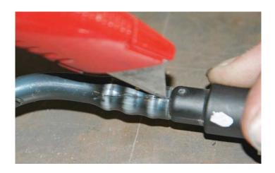
174. Remove the end fittings from the plastic tubing.
