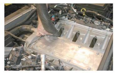
51. Cover the intake manifold ports with tape or clean rags to keep dirt and objects from entering the engine.
