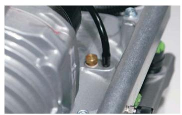
203. Connect the remaining end of the hose to the Fuel Pump Booster vacuum barb located on the side of the unit. Secure the hose out of the way with the Ty-wraps supplied.
