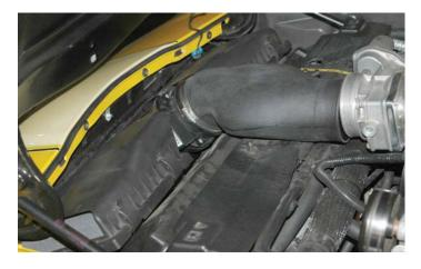
170. With the air tube and filter assemblies in place, install the black coupling hose and clamps on the end of the air tube to meet the throttle body. Tighten the clamps securely.
