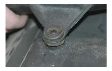
26. Remove the air filter assembly complete with the MAF and bellows from the vehicle.
