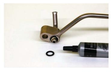
109. Install the new vent pipe with the original bolts and torque them with a torque wrench and 10mm socket to 106 in-lbs
