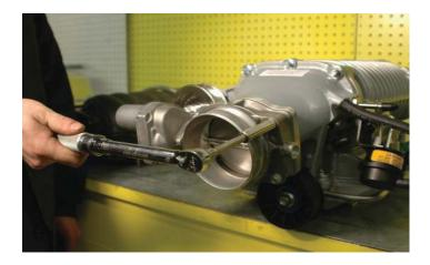
142. Remove the Manifold Absolute Pressure (MAP) sensor from the stock intake manifold by tilting the sensor forward and lifting it free. Ensure that the orange rubber seal is not missing or damaged as it and the sensor will be re-used.
