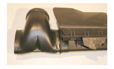
166. Install a gasket onto the Mass Air Flow meter (MAF) and note where the "Tooth" contacts the gasket.
