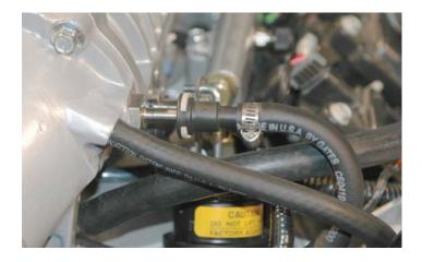
178. Connect the original EVAP hard-line to the upper barb of the solenoid and re-connect the solenoid electrical connector.
