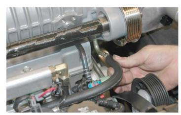
183. Connect the vehicle fuel line to the barb on the fuel manifold by pushing it on firmly.
