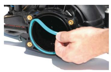
140. Install the throttle body gasket into the groove on the supercharger inlet manifold.
