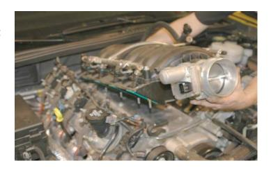
50. Using a vacuum cleaner, remove any dirt or debris from the intake port area. (Be careful not to get any debris in the intake ports.)
