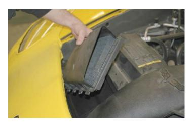
24. Loosen the air filter bellows clamp with a 6mm nut driver or a straight blade screwdriver.
