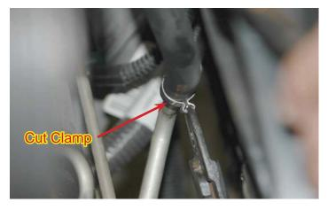
133. Route the new hose from the small barb on the PS reservoir along the same path as the 5/8" hose and trim it to length. Connect the hose securely to the hard line with the #4 clamp supplied. Using only GM recommended fluid, fill the power steering reservoir to the full cold mark. (Recheck the level after start up and after turning the steering wheel lock to lock a few times.)
