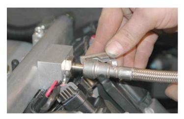
185. Insert the new brake vacuum check valve into the end of the 11/32" vacuum hose supplied.
