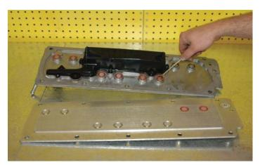
115. Install the new valley cover and flathead bolts supplied with a 5mm Allen socket and torque wrench. Torque the bolts to 15 ft-lbs. Insert the six O-rings supplied in the recesses in the valley cover.
