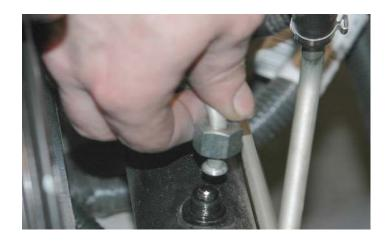
74. Replace the sway bar by installing it in its original position and replacing the sway bar brackets and reconnect the end links.
