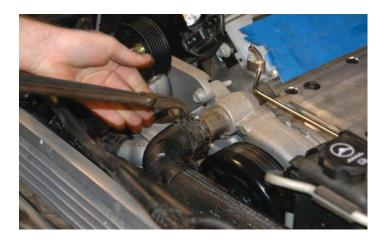
118. Using a power steering oil suction tool or turkey baster, remove the fluid from the power steering (PS) reservoir and put into a disposable container. (Old fluid can be disposed of an a oil recycling center.)
