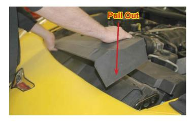
22. Remove the air filter hood clips on both air filter elements .
