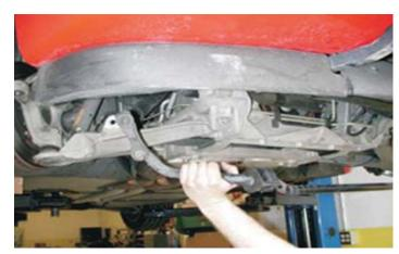
55. Remove the fan assembly by pushing up on the fan shroud to Un-clip it from the radiator and then pull the assembly out from the vehicle completely.
