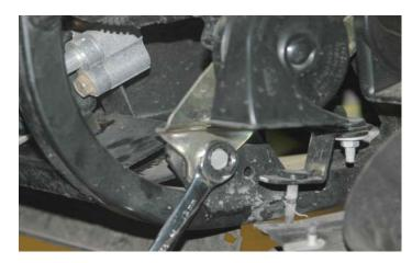
83. Squeeze the electrical connector on the horn assembly to disconnect it.
