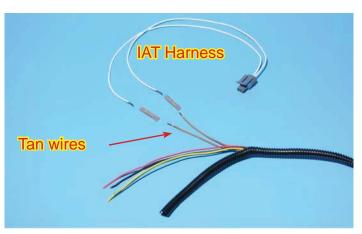
215. Extend the remaining three wires of the MAF harness using the supplied color coded wire and crimp/shrink connectors to connect to the MAF connector. (Note that the two tan wires on the MAF connector will no longer be used.) Cover the extended harness and the new IAT branch with the split loom supplied.
