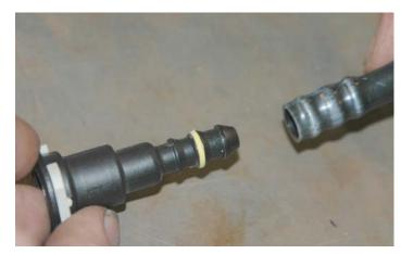
175. Using a 18" length of the 5/16" hose provided, insert the EVAP end fittings into the end of the hose and secure them with the #4 clamps provided.
