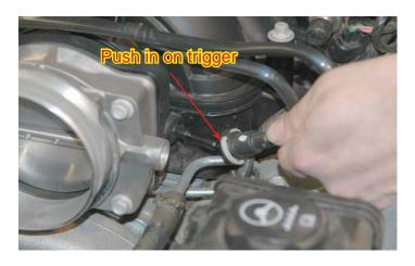
34. Release the other end of the tube at the bottom of the EVAP solenoid by pushing in on the release trigger.
