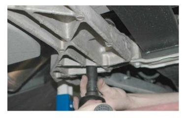
77. Torque the sub-frame, sway bar connections and motor mounts to the torque values below: Torque Specifications:
