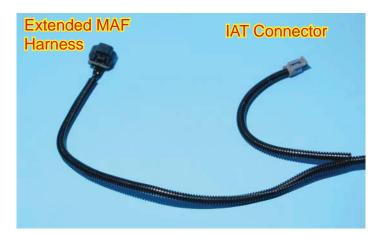
216. Route the IAT harness under the fuel rail and plug the IAT connector into the IAT sensor.
