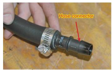
123. Install the 5/8" hose with the connector into the end of the large PS hose to the pump. Secure the connector with the original spring clamp.
