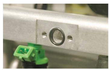
147. Next install the fuel manifold to the fuel rail using the supplied Allen bolts. Tighten and torque the bolts with a 4mm Allen socket and torque wrench.
