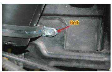
88. Secure the clamp bolt on the bottom of the panel with the nut and washer supplied. Tighten them with a 10mm wrench
