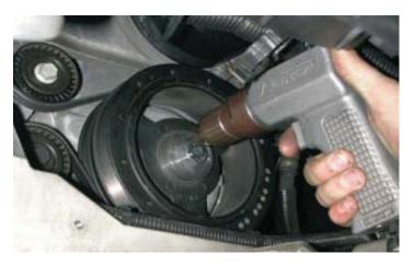
68. Using a 24mm socket, remove the large bolt and the drill guide from the engine.
