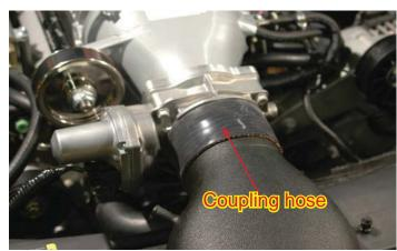
171. Using the length of 3/8" PCV hose supplied, connect one end to the barb on the upper air tube. Note: The coupling hose clamps in place.
