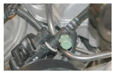
179. Connect the remaining end of the EVAP hard-line to the original firewall connection.
