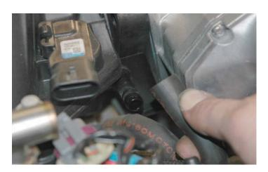
48. With a 8mm socket wrench remove the ten intake manifold bolts.
