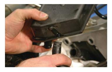
122. Using the length of 5/8" hose supplied, install the hose connector in the end of it and secure it with the #10 clamp supplied.
