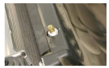
95. Remove the center bolt in the spoiler with a 10mm socket wrench.
