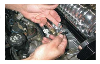
152. Torque the supercharger manifold bolts, working from the center out to 89 In-Lbs. (10 Nm) using a 10mm socket and a inch pound torque wrench.
