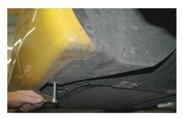
9. Removing the inner fender panel will expose the vehicles operating computer.
