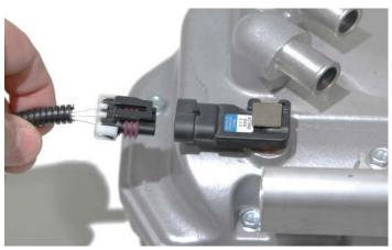
213. Locate the MAF sensor connector and peel back the tape and split loom to expose the wires. Approximately 3" from the connector cut all the wires.
