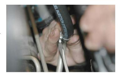
134. Using a pair of pliers to squeeze the stock spring clamp, rotate the coolant line shown where it meets the water pump housing. Rotate the hose so that it will not contact the tensioner mounting bolt and release the clap to hold it the new position.
