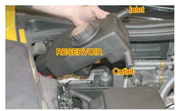
99. Using the length of 3/4" hose supplied, install one end on the outlet barb of the reservoir and route it under the fuse relay center and along the frame down to the coolant pump. The complete routing of all the hose is shown.
