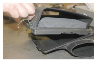
159. Remove the paper air filter elements and use a shop towel to remove any debris.
