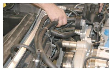
131. Connect the 5/8" PS hose to the large barb on the bottom of the PS reservoir and secure it with a #10 clamp supplied. Replace the upper radiator hose into its original position.
