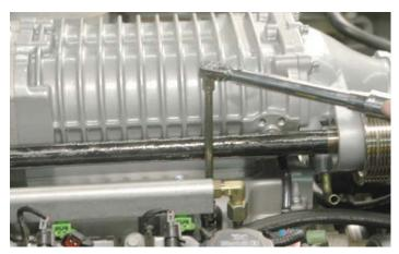
153. Install the new supplied supercharger and accessory fan belt with a 15mm tensioner wrench, using the new supplied belt routing diagram below.
