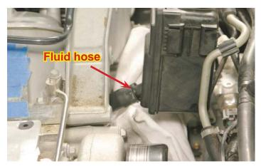
121. Remove the small hose from the bottom of the reservoir and set it aside for re-mounting in a later step.
