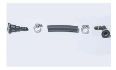
176. Connect the end of the new EVAP line with the right-angle "elbow" fitting to the lower barb of the EVAP solenoid.
