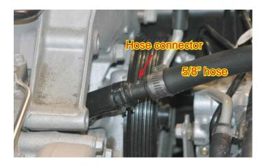
124. Pass the 5/8' PS hose through the center of the new serpentine drive belt.
