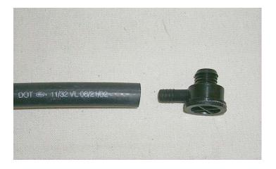
186. Install the check valve and hose assembly into the grommet on the power brake booster.
