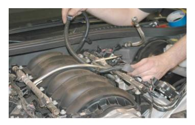
46. Remove the power brake check valve and hose from the brake booster grommet by pulling it out firmly.
