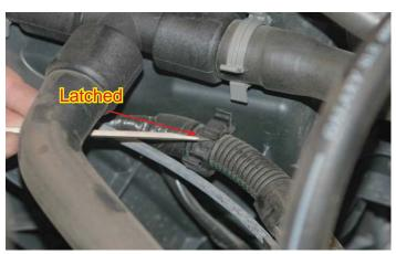
31. Locate the cooling fans electrical connector under the wiring harness located on the fan shroud. Squeeze the connector firmly and pull the connector free as shown.
