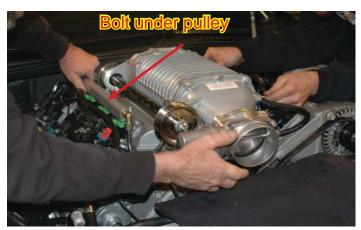
151. Remove the black plastic sleeves that hold some of the intake bolts up and start all ten intake bolts by hand. Do not tighten until all the bolts are started. (Be careful not to cross thread the bolts.)
