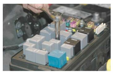
199. Replace the positive battery cable on the (B+) terminal. Install the ring connector of the larger red wires from intercooler relay on the B+ terminal. Reinstall the nut and tighten it securely with a 12mm wrench. Replace the Fuse/Relay center cover.
