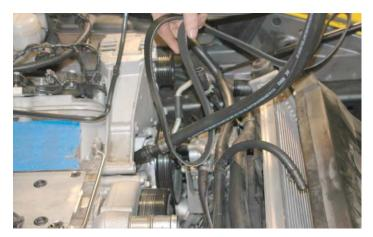
125. Re-install the mounting bolts back into the alternator bracket and tighten to 50 Nm (37 ft-lbs).
