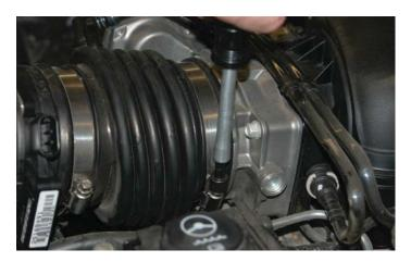
25. Lift straight up on the plastic air tube to detach it from the two locating pegs.
