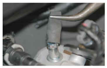
181. Assemble the PCV outlet hose by cutting a 2" length and attaching one end to the 90 degree "Elbow" fitting. Attach the other end to the barb on the driver side valve cover. From the remaining length cut a 38" length and connect one end to the remaining barb on the elbow fitting.
