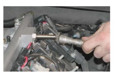
184. Secure the fuel line by re-installing the safety clip.
