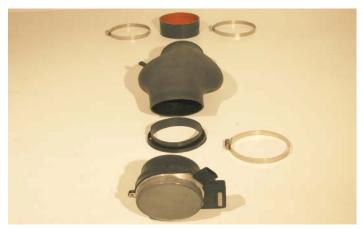
169. Assemble the upper air tube assembly onto the lower and install themon the vehicle as shown.
