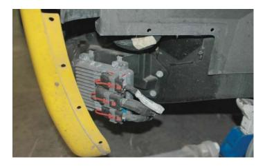
10. There are three computer connectors, Grey, Black, and Blue. Remove the connectors by first removing the Red locking key, then pushing in on the Black cover and pushing the Grey latch down.
