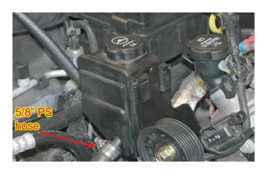
132. Locate the small hose removed from the PS reservoir and follow it down to where it connects to a hard line. Cut the clamp securing the hose to the hard line and remove the hose.
