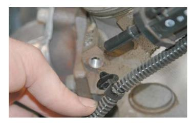
127. Install the new PS reservoir mounting bracket using the new bolts supplied. Tighten the bolts securely and torque them with a 15mm socket and torque wrench.
