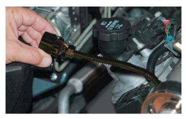
208. Plug the provided ETC extension harness into the existing ETC plug and route under the supercharger nose to the driver side of the vehicle.
