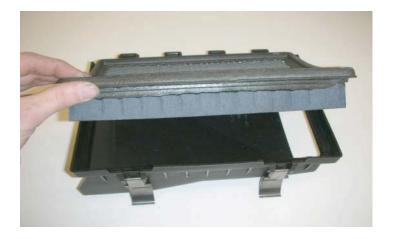
162. Install the new air filter elements and re-clip the hoods onto the filter boxes.
