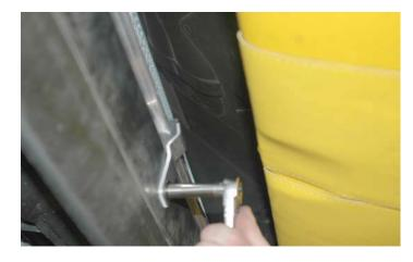
97. Using the 1" hole saw again, create one or two holes in the right hand splash panel below the radiator. This is where the coolant lines will pass through to the heat exchanger.
