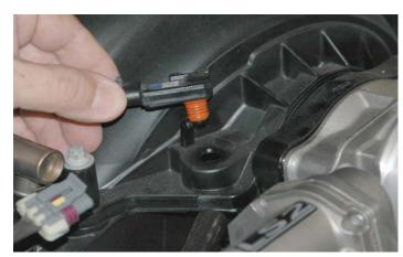
143. Apply a small amount of the grease supplied to the MAP sensor seal and install the sensor in its new location at the right rear of the supercharger manifold.
