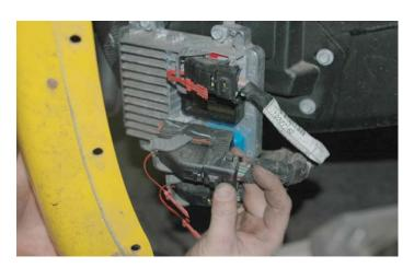
12. Note: If your vehicle has a automatic transmission, you will also need to remove the transmission control computer located on the back side of the mounting bracket.
