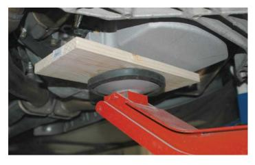
61. When raising the engine with the floor jack, take care to watch the clearance between the back of the engine and the fire wall, so as not to damage any of the components on the fire wall.
