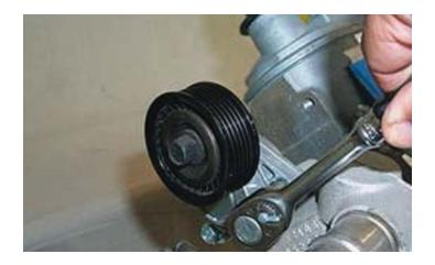
106. Install the new tensioner assembly in place of the stock unit with the original bolts and torque them to 40 ft-lbs.
