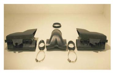
164. Install the gaskets onto the inlets of the lower air tube assembly as shown
