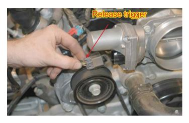
40. Disconnect the Manifold Absolute Pressure (MAP) sensor connector.
