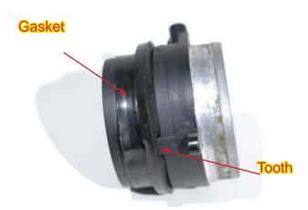
167. To allow the gasket to seal better around the MAF, mark then cut with a shop knife a notch in the gasket 7/16" (11mm) wide by 1/4" (6mm) deep in the inside edge using the tooth as a guide.
