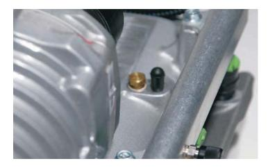
202. Using the hose supplied, connect one end of the hose to the pressure port and then route the other end to the Fuel Pump Booster module. Secure the hose out of the way of the rotating parts at the rear of the blower with the Ty-wraps supplied.
