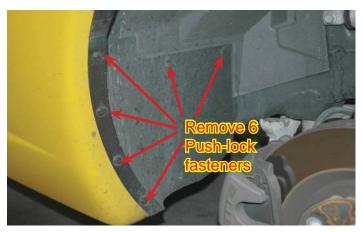
7. Remove the Push-lock fasteners by gently prying up on the center of the fastener and then removing the fastener completely.
