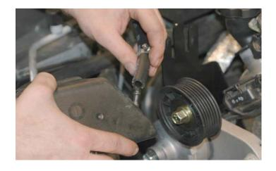
129. Slide the PS reservoir into place on the new mounting bracket.
