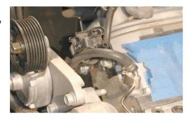
138. Remove the throttle body from the plastic intake manifold with a 10mm socket wrench.
