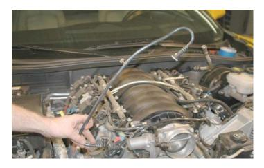
36. Release the vent tube at the top of the EVAP solenoid by pushing in on the release trigger.
