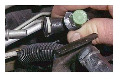
180. At the rear of the driver side valve cover, remove the rubber cap on the valve cover barb.
