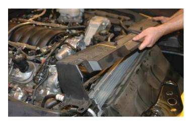
29. Un-clip the coolant hoses from the fan shroud.
