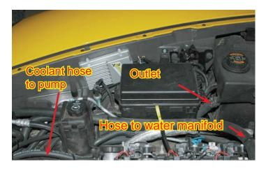
100. Cut the hose to length and connect the hose to the inlet barb of the pump. Secure both ends of the hose with the spring clamps supplied.
