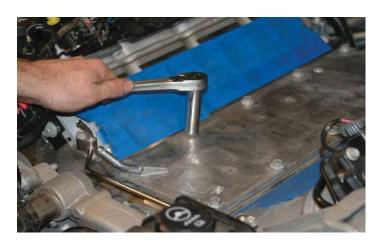
113. The gasket will be reused, the original valley cover will not. Inspect the gasket for any damage and then re-install, note that it will only fit correctly in one position.
