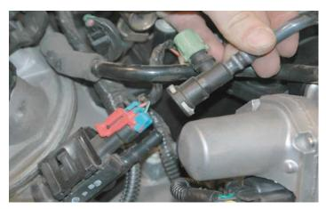
37. Disconnect the EVAP solenoid electrical connection.
