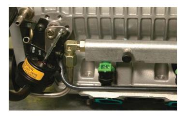
150. Carefully, set the supercharger assembly on the engine, line up the bolt holes with the holes in the cylinder heads. (Be careful of the one bolt that under the rear supercharger pulley on the passenger side as it protrudes and must be aligned first.)
