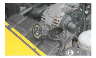
222. Temporarily lift the intercooler reservoir out of the way to re-connect the battery ground terminal.
