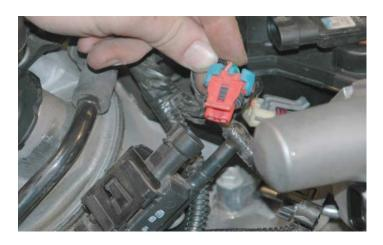
38. Disconnect the vent tube at the fire wall connection and set it aside as it will be reused in a later step.
