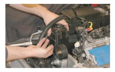
130. Route the 5/8" PS hose along the fan shroud, following the same path as the coolant lines.
