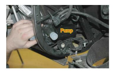
87. The small panel the pump will mount on has a hole in it near the front edge. Pass the bolt for the mounting clamp through this hole.
