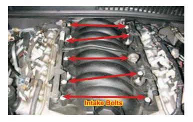
49. Carefully remove the intake manifold and set it aside.
