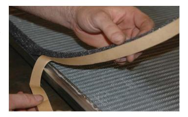
90. Apply a small piece of the foam strip to the Heat Exchanger Retaining Bracket.
