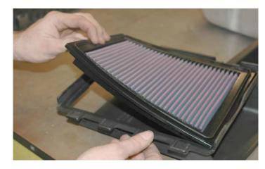
163. Here is a dismantled view of the new inlet assembly. Note: The new lower air tube and gaskets.
