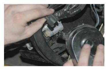
84. Use a 10mm wrench to remove the nut that secures the bottom edge of the nose cover.
