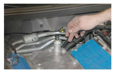
111. Use a 1-1/16" socket wrench to remove the oil pressure sensor from the engine valley cover.
