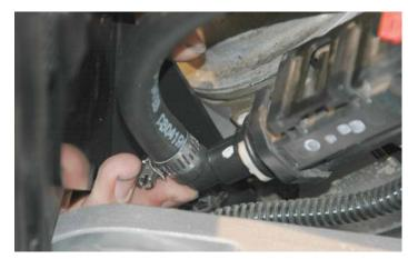
177. Connect the remaining end of the new EVAP line to the barb on the driver side of the inlet manifold.
