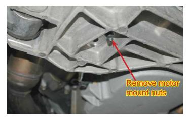
59. Using a suitable pry bar, pry down the subframe at the front two mounting points. Temporally push a metal or wooden wedge approximately 3/8" thick between the frame and sub frame at these points.
