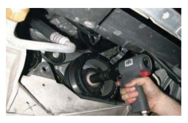
64. Install the drill guide using the supplied bolt and tighten to 30 ft-lbs with a 24mm socket and torque wrench.
