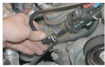
35. Remove the tube completely and set it aside as it will be re-used in a later step.
