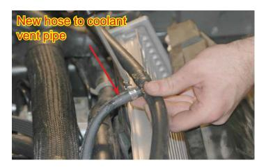
137. Connect the hose from "T" fitting to the barb on the coolant vent pipe. Secure the hose with the #4 clamp provided.
