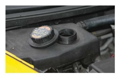
224. Using a straight blade screwdriver. Open the bleed valve to let any trapped air escape form the intercooler system. Some coolant will be lost when bleeding the system. Add coolant as necessary to the reservoir and continue to bleed the system until you can get a steady stream of coolant from the valve for over one minute. Check the intercooler reservoir level and re-open the bleed valve as needed.
