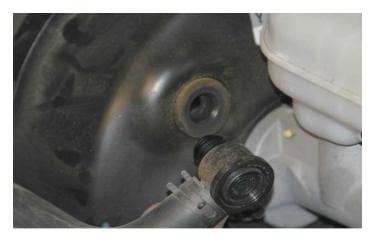
187. Cut the power brake hose to length and connect the remaining end of the hose to the barb on the driver side of the inlet manifold.
