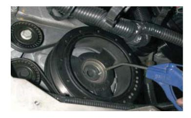
70. Insert the two supplied hardened roll pins into the drilled holes. The use of a small hammer and punch may be necessary to tap the pins in. (Make sure that the pins are in far enough that they do not touch the balancer bolt.)
