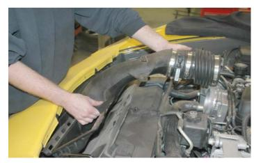
27. Using a 10mm socket wrench, remove the two bolts on each side of the radiator cover.
