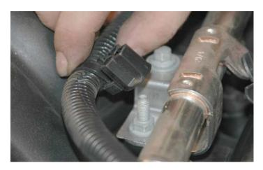
45. Free the battery cable from the intake manifold and lay it aside.
