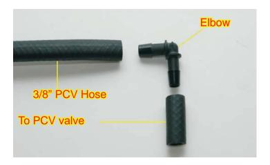
182. Connect the remaining end of the PCV hose to the 3/8" hose barb located on the bottom of the bearing support for the supercharger drive shaft.
