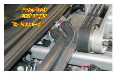
156. This is a plumbing diagram for the intercooler system. Note: The final connections for the intercooler will be made in a later step.
