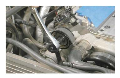
105. Remove the stock tensioner assembly by removing the two mounting bolts with a 15mm wrench.
