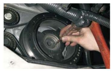
71. Install the new supplied factory GM harmonic balancer bolt.
