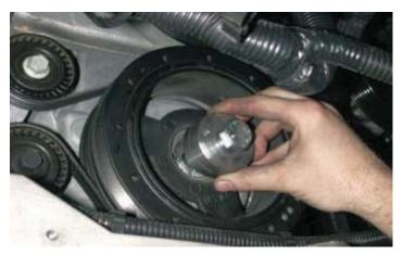
69. Use compressed air to blow out the holes.
