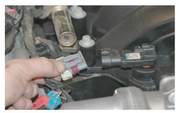
41. Use a shop knife to cut the tape that secures the wiring harness to the fuel rails in four locations.
