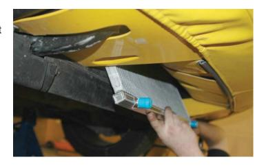
94. Move the heat exchanger around until the air-bleed valve appears in the newly created hole in the radiator shroud.
