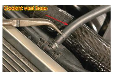
136. Connect the new 1/4" coolant hose to the coolant vent "T" fitting with the #4 clamp supplied. Tighten the clamp securely and route the hose along the same path as the PS hoses to the barb on the coolant vent pipe. Replace the radiator cover previously removed.
