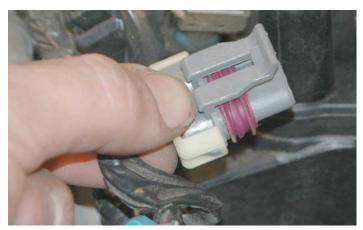
211. Install the new MAP harness to the original wires using the crimp/shrink connectors supplied. The new harness wires are all white, so care must be take so the new white wires are in the same positions as the colored wires on the original connector. Strip about ¼" of insulation from the ends of all the wires. Crimp the connectors on and shrink the insulation so that it contracts around the wires completely.
