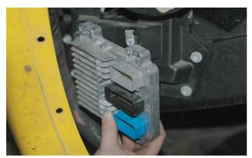
219. Replace the computer connectors in their original positions, making sure to lock them in place by pushing the grey levers towards the harness. Secure the connectors by inserting the red lock keys in position.
