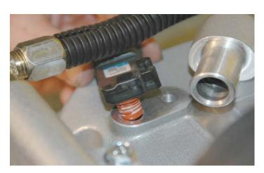
144. Install the MAP sensor in its new location using the supplied bracket and the button head Allen screw with a 4mm Allen wrench.
