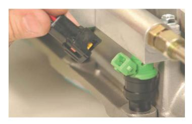
207. Locate the Electric Throttle Control (ETC) connector on the passenger side of the vehicle near the oil fill spout.
