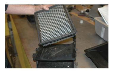
160. California spec cars only: Ensure that the Vapor Elements inside the filter boxes are intact. Do not remove them!
