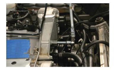
126. Remove the wiring harness anchor from the front of the right (passenger side) cylinder head.
