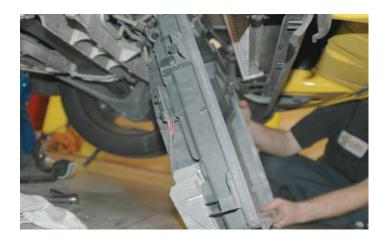
76. Remove the wedges from between the frame and sub frame. Tighten the sub frame and motor mount nuts securely.
