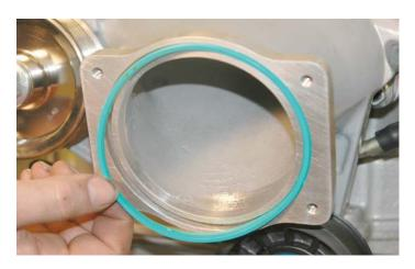
141. Install the throttle body onto the inlet manifold using the original bolts. Tighten the bolts with a 10mm socket and torque wrench to 106 In-Lbs (12Nm).
