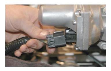
210. Locate the Manifold (ETC) connector and peel back the tape and split-loom to expose the wires. Cut the wires approximately three inches from the connector.
