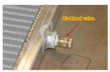
92. Using a 1" hole saw, make a hole in the top of the radiator shroud on the passenger (right) side. This will create a access hole for the coolant air-bleed valve.
