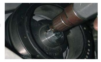
66. Using compressed air, blow the drill shavings out of the holes.
