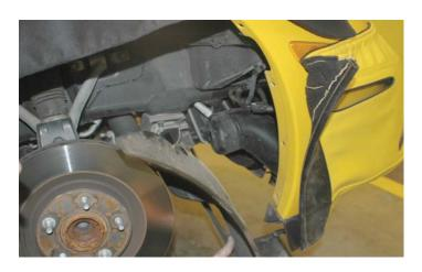
81. Remove the brake cooling duct, it will pull out.
