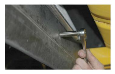
96. Install the Heat Exchanger Retaining Bracket with the bolt removed in the previous step. Ensure that the foam pad is contacting the lower tank of the heat exchanger and tighten the bolt securely.
