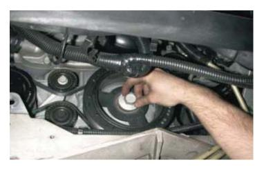
72. Using a 24mm socket tighten the new harmonic balancer bolt according to General Motors specifications. Tighten to 50 Nm (37 ft-lbs) then tighten an additional 140 degrees using a torque angle meter.
