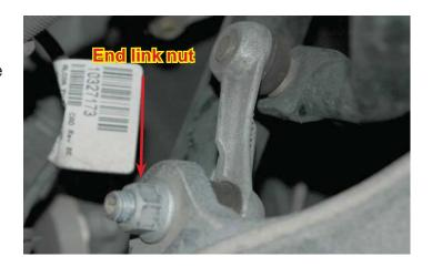
54. After removing the sway bolts, brackets and end link nuts, remove the sway bar and set it aside.
