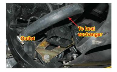
102. Cut the hose to length and then install the 90 degree "elbow" fitting into the end of the hose. Cut a three inch length of hose from the remaining hose and connect it to the elbow fitting. Finally connect the 3" length to the driver side barb of the heat exchanger. Secure all connections with the spring clamps supplied.
