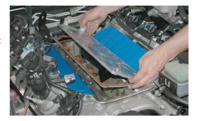
114. From the bottom of the original valley cover, remove the eight O-rings with a small straight blade screwdriver. Install the O-rings into the grooves in the bottom of the new valley cover.
