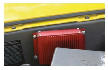
201. On the driver side (left) rear of the supercharger manifold, locate the pressure port capped with a small, rubber cap and remove the cap.
