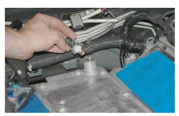
112. Use a 12mm socket wrench to remove the ten bolts that secure the engine valley cover.
