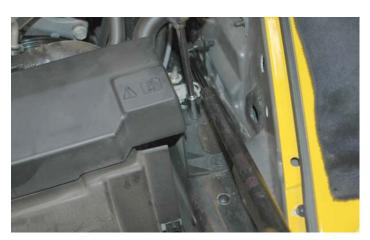
28. Remove the radiator cover and set it aside for a modification in a later step.
