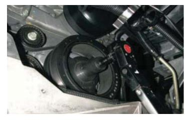
65. Using a small or angled 3/8" drill and the supplied drill bit, insert the drill into the guide holes and drill to the second step of the drill bit. (Make sure that you drill all the way to the second step.)
