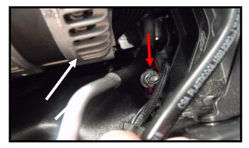
On Z51 cars you can use the 10mm bolt on top of the oil tank for the ground wire. Non Z51 cars, route the black wire along the plastic piping going towards the alternator (white arrow). Secure black wire on the ground terminal below the alternator (red arrow) using the supplied nut. This is where a magnet comes in handy. Its easy to drop the nut.
