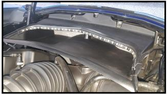
Now you can mount the hood vent strip. Wipe the mounting area with the supplied alcohol pads. Apply the adhesion promotor to the edge of the ducting. Position the strip as shown. Center the strip on the ducting so the wire comes out as shown in the next picture. Be sure to work the strip into the center and corners as this is the most likely place for it to want to pull off. Keep working it until it fits the corners well.
