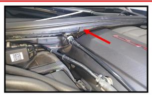
After the strips are mounted you can hide the cable behind the heat shield under the cowl lip on the passenger side. Tuck the cable under the shield all the way over to the drivers side.
