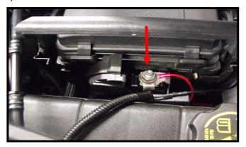
Install the red loop over the positive connection and use supplied nut and tighten. Keep in mind where you want to mount the box and route your wires accordingly. You can re-route them later to hide wires.
