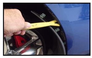
Turn the wheel out on the side you're working on. Use a pry tool to pop the front splash guards out. There is also a screw underneath if you want to take it all the way off. Repeat on both sides.
