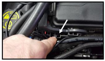
To gain access to the positive connection release these tabs on each side of the rear of the fuse box while raising the handle. Release the cover over the positive terminal
