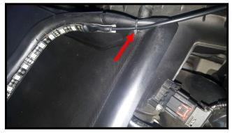
To secure the wire in place drill a 1/8" hole in the ducting below the wire and use a wire tie to secure the wire to the ducting. You can use more than 1 tie if you wish.
