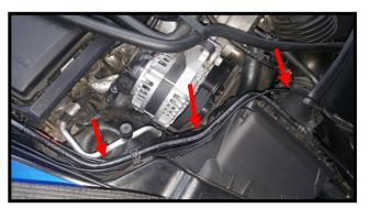
Route the wire along this tubing toward the connectors on the control box. Secure with wire ties.
