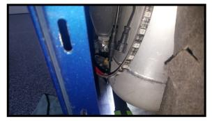
This shows the led strip and extra lead inside the fender cove. The extra lead is to connect the rear fascia kit if you are installing it. Use bungie cords to keep fender shield pulled back.
