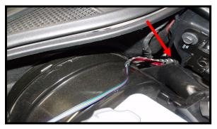
Feed the drivers side led strip past the brake booster and down into the area where you placed the light.
