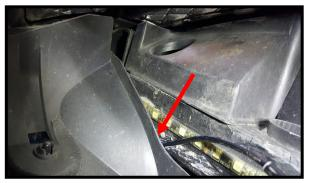
Route the led cable through any opening on the passenger side of the air box. It will come out below the wiring harness below the hood hinge assembly in the engine compartment.
