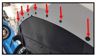
Raise the front of the car so you can get at the fascia screws. Remove the seven 8mm screws. (red arrows). Also remove the  $4 \times 10$ mm bolts at the rear of this same panel and slide it rearward to remove it.
