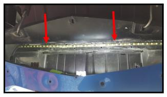
Cut the very top off the adhesion packet. Squeeze the excess fluid back into the packet as you remove it. Fold the top over and seal to preserve the remaining fluid for use on other kits you may have purchased. Center the strip in the grill opening and mount it to the bar as shown. Tape the wired end down with duct tape.
