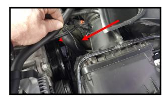
Find where the led wire came through in the engine compartment and route the wire under the air filter housing and up by the alternator. Route the cable towards the extra lead on the control box using the same path as the hood vent cable.
