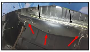
Next remove the 4 screws that hold the front of the lower radiator shroud. (red arrows). This panel is very flexible so pull it back and secure with bungie cords as shown. You can see where the LED strip mounts (black arrows).
