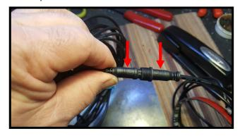
Pull back the nut on the connector on the control box so you can see the arrows. Line up the arrows and connect the cable with the plastic nut. Test the led strip. Secure the wires away from the alternator or any moving parts with the wire ties. Once everything is working you can re-assemble the panels you took off by reversing the removal procedures.
