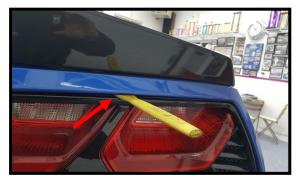
Insert a plastic removal tool between the tailight bezel and the rear fascia. The next picture shows the tabs you are releasing. Pull out on the bezel as you work your way around . Remove both.
