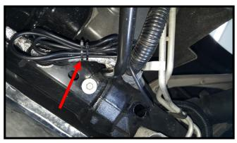
Now go back and tape down the cables wherever you can. We tape them to the bottom of the rear fascia where the cables go out to the side vents. Wipe the panels first as they will be dirty. Finally bundle the extra cable and tie it up away from the exhaust system.
