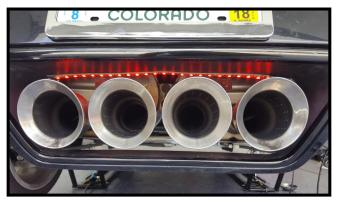
Wipe the front most edge of the area over the tailpipes with alcohol pads then apply a thin coat of adhesion promotor. Reseal packet so it doesn't dry out. Center the exhaust strip and attach it along the front most edge as shown. Always route cables away from the exhaust.
