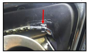
Remove the backing from the cable clips before you stick the ends of the led strips. Be sure to prep this area with adhesion promotor. Come back and press the clips in place after a few minutes.
