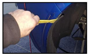
Pry both rear splash guards out. Remove the  $2 \times #15$  torx screws. Pull the fender shield back and bungie cord back so you can see inside the quarter panel.
