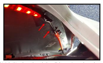
This is looking down through the tailight opening to show where to mount the side led strips. Mount them a couple inches forward of the vents. Wipe with alcohol then apply adhesion promotor sparingly. Center the strips in the openings and peel the backing off to apply. Always tape the cables to the panel to prevent the strips from pulling off. (red arrows). Repeat on both sides.
