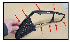
There are 3 on the top and bottom, 3 on the wide side and 2 on the narrow end. Pull out as you release the tabs.
