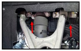
There are 2 holes in the frame you can use to isolate the wire from the wheel area. You can use a coat hangar to tape the wire to and fish from one hole to the next. You could also wire tie the cable to the wiring below the holes but it wont be as protected. You can also fish it to the hole in the next picture which is on the bottom of the frame further back.
