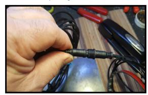
Line up arrows on the connector and plug it in to the extra lead by the front cove led strip. Tighten the nut.
