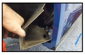
The inner fender panel is very flexible so you can untuck it from behind the fender then lift the bottom up and out to gain access to the rocker panel area to fish the extension cable from front to rear.
