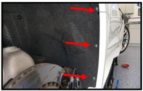
Raise the vehicle and remove the right rear wheel. Remove the 3 #15 torx screws. There is 1 x 7mm screw underneath to remove also. Remove the front wheel splash shield and #15 torx screws if you haven't already.
