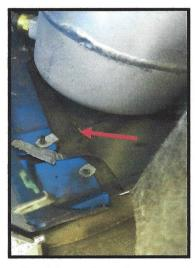
Using a long stiff wire (straightened coat hangars taped together works), feed the wire all the way from the back to the front cove area. Wire will come out at the bottom of the inner front fender. Tape the end of the extension cable with the nut on it to the fishing wire and pull it through to the back
