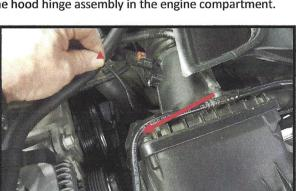
Find where the led wire came through in the engine compartment and route the wire under the air filter housing and up by the alternator. Route the cable towards the extra lead on the control box using the same path as the hood vent cable.
