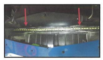
Cut the very top off the adhesion packet. Squeeze the excess fluid back into the packet as you remove it. Fold the top over and seal to preserve the remaining fluid for use on other kits. Center the strip in the grill opening and mount it to the bar as shown. Tape the wired end down with duct tape.
