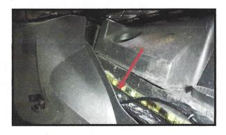
Route the led cable through any opening on the passenger side of the air box. It will come out below the wiring harness below the hood hinge assembly in the engine compartment.
