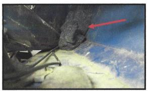
Looking toward the front of the car in the dark recess you just uncovered there are 2 wads of stuffing that need to be removed. They are stuffed into the rocker panel area to block debris so you may have to reach way in to grab them.
