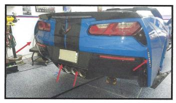
Lay out the rear kit with the connection lead on the passenger side. Lay the center exhaust section on top of the tailpipes and route the side led strips behind the fascia and out towards the tailight openings hanging the short led strip out of the tailight opening. Place a light behind the lower rear vent so you can see where to route the leds. Line up the arrows on the connector and test before mounting leds.
