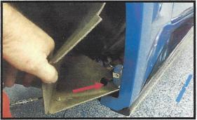
Route the cable at the back through the hole in bottom of the fender panel.
