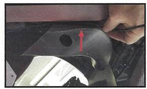
Route the wire behind the brake scoop up towards the frame.
