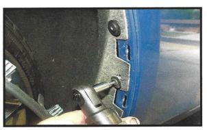
Use a # 15 torx to remove the 3 screws behind the splash shield. Pull back the inner fender panel to get to the cove area. Place a light inside the fender to guide the led strips in place.
