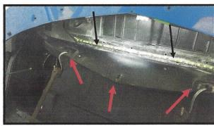
Some cars will have an oil cooler here. If so, remove the 2 bolts on each end and swing it out of the way. Otherwise remove the 4 screws that hold the front of the lower radiator shroud. (red arrows). This panel is very flexible so pull it back and secure with bungie cords as shown. You can see where the LED strip mounts (black arrows).
