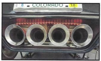
Wipe the front most edge of the area over the tailpipes with alcoho pads then apply a thin coat of adhesion promotor. Reseal packet so it doesn't dry out. Center the exhaust strip and attach it along the front most edge as shown. Always route cables away from the exhaust.
