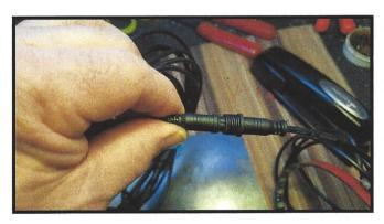
Pull back the nut n the controller connector so you can see the arrow. Line up the arrows and slide the connector together and tighten the nut. Test the lights again.
