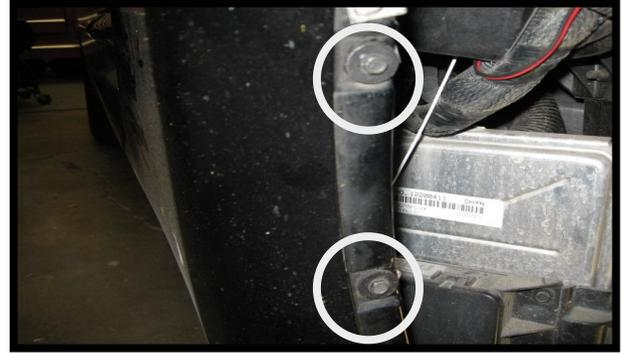
Remove these 2 x 7mm screws and remove the cove shield Now is a good time to paint the cove shields so they can dry.
