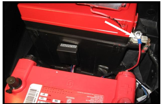
Now slide the cover off the fuse box positive terminal (white arrow). Connect the red wire to this terminal using the supplied nut. You can also connect it to the battery.
