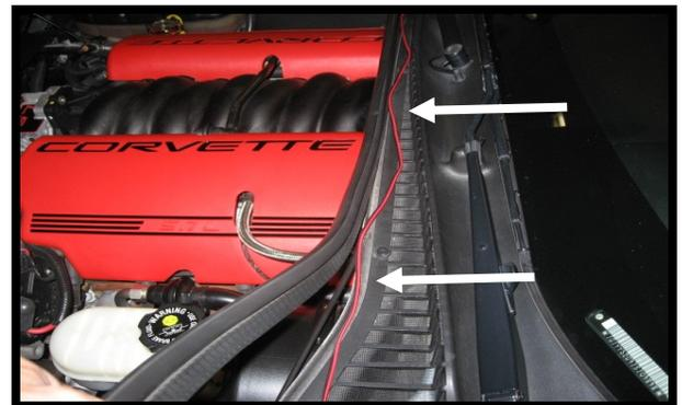
Next pull the cowl weatherstrip off by pulling it forward. Route the long led wire across the cowl to the drivers side hood latch area. You can also run the wires behind the engine away from exhaust.
