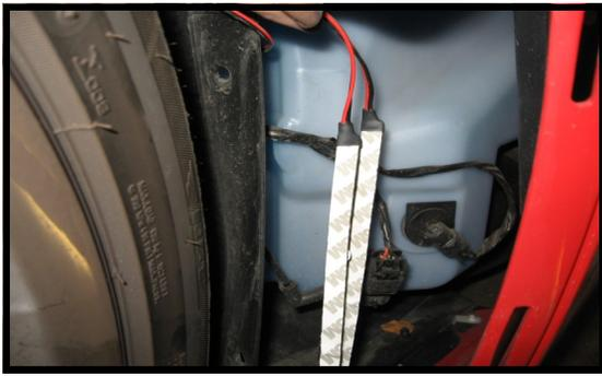
On the drivers side, drop the leds past the washer reservoir & into the cove area. Wipe mounting area with alcohol pads. The best light pattern is achieved by placing the strips about 1" back from the rear edge of the opening facing the shield. Hold strips in place firmly for a minute.
