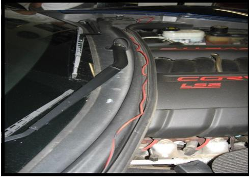
Place the remote control box by the battery and stretch the long led wire across the cowl. Pull the cowl weather strip off by pulling forward on it.
