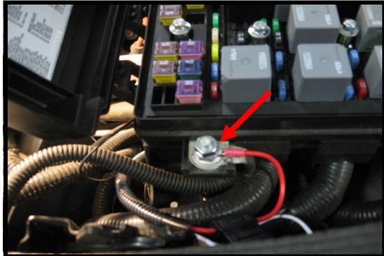
Open the cover over the + battery connection at the under hood fuse box. Place red wire from control box over this stud and secure with provided nut.
