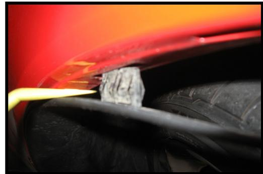
Using a panel removal tool and a shop rag to protect paint, pry between the panel and fender to unlatch these clips. The one at the top of the fender has a hooked retainer so remove the 2nd and 3rd ones first
