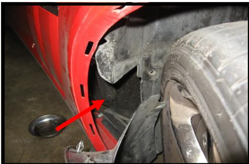
Shield removed to gain access to cove area. Leds will drop into this area for installation.
