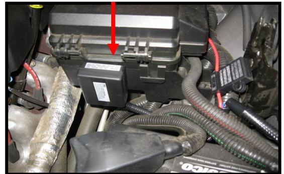
After all wires are secured and lights are working, You can now mount the control box. The box is not water-proof so cover when washing engine compartment. You can now re-assemble all shields. Remember, the Inner fender panels have a hooked clip on the top that should go in first. Enjoy the new lights!!
