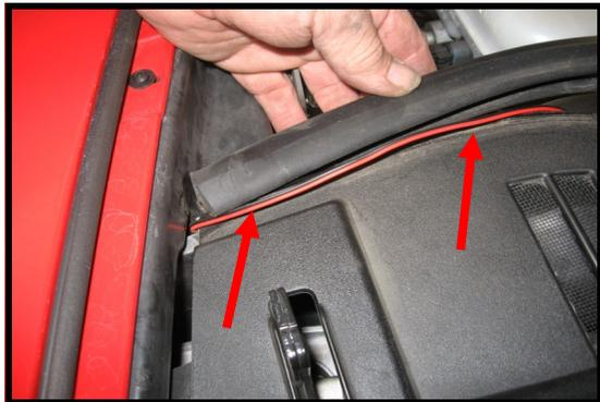
Secure the wire across the cowl by inserting it into the weatherstrip and pressing the strip back in place across the cowl area.
