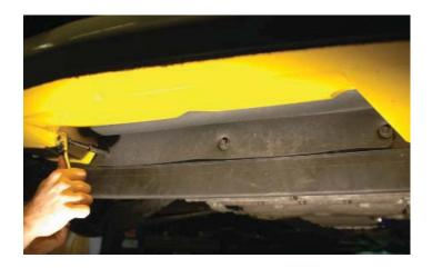
254. Place a strip of light colored tape on the driver side of the upper grooves in the splash shield/air deflector in front of the radiator/heat exchanger as shown.
