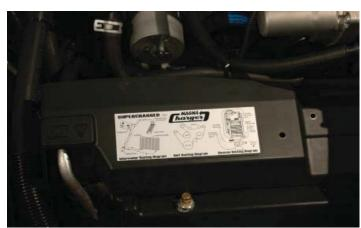
284. Affix the OBDII port cover on the OBDII port at the driver side below the dash. Clip the cover ring on an adjacent wire to keep it local.
