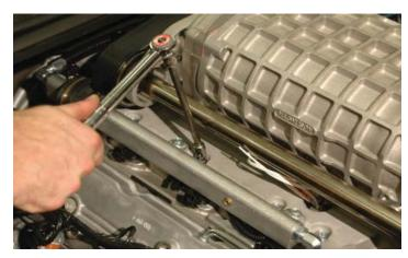
155. Use a 14mm wrench to remove the idler pulley directly below the supercharger inlet.
