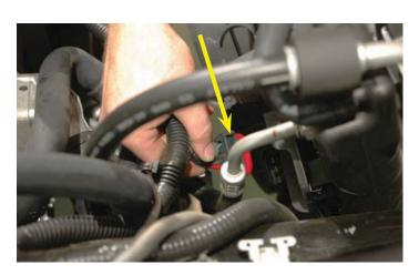
56. The fan shroud is held to the radiator by two bolts. One is located near the bottom of the radiator on the driver side. The other is located high on the passenger side. Use a 10mm wrench and remove this bolt.
