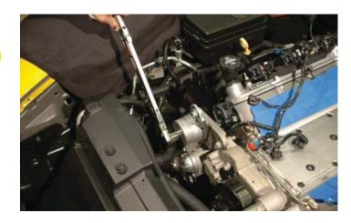
116. Place the other angle from the tensioner brace bracket package on the back of the long bolt you just tightened. The Long slot should align with the long slot on the angle mounted earlier on the power steering reservoir bracket. Tighten in place aligning the two angles together. Use the provided nut and bolt to tie the two angles together, anchoring the tensioner assembly.
