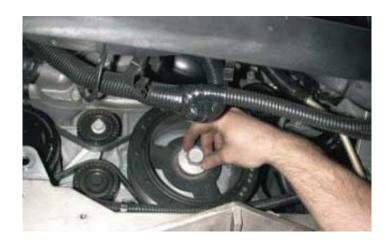
78. Using a 24mm socket tighten the new harmonic balancer bolt according to General Motors specifications. Tighten to 50 Nm (37 ft-lbs) then tighten an additional 140° using a torque angle meter.
