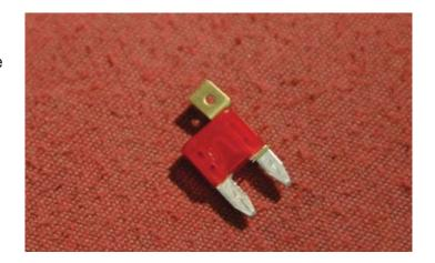
234. Re-install the fuse with the fuse-tap back in the original location.
