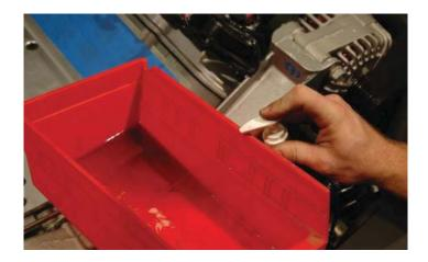
102. Using a 15mm wrench, remove the two bolts that secure the power steering fluid reservoir to the alternator bracket.
