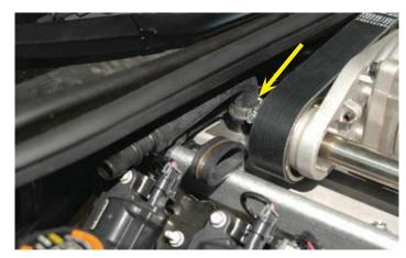
213. Cut 2" off of the short end of the other supplied ¾" x 4" x 18" elbow hose. Cut the long end off to fit where it will join the hose you just installed on the supercharger intercooler. Use the supplied spring clamps on the coupling end and worm gear clamps on the reservoir end and supercharger inlet end. Tighten firmly.
