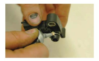
146. Install the sensor in its new location at the passenger side rear of the supercharger manifold and drop the split-loom spaced bolt into the mounting hole.
