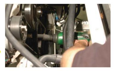
70. Install the drill guide using the supplied bolt and tighten to 30 ft-lbs with a 24mm socket and torque wrench. Orient the holes to give you access with your drill. We found 2:30 and 8:30 worked pretty well for us.
