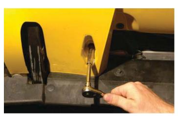
248. Bolt the brake cooling duct back to the original location in the wheel well using the stock hardware, and insert the push pin rivet back in the front to cowl splash shield location.
