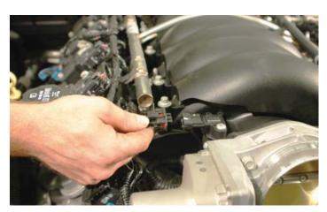
32. Use a shop knife to cut the tape that secures the wiring harness to the fuel rails in four locations.
