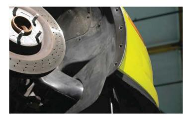
250. NOTE: For vehicles with the soft rubber air deflector follow the next four steps. If your nose fascia was attached in step #247, skip to step #254. Re-attach the underside ends of the nose fascia as shown using the two outside 7mm bolts, tighten securely.
