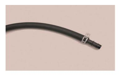
120. Install the 5/8" hose with the connector into the end of the large power steering hose to the pump. Secure the connector with the original spring clamp.
