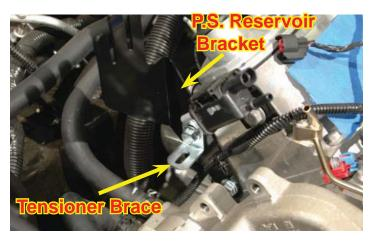
108. Cover your engine well, as we will need to do some sawing and grinding for clearance with the new tensioner assembly.
