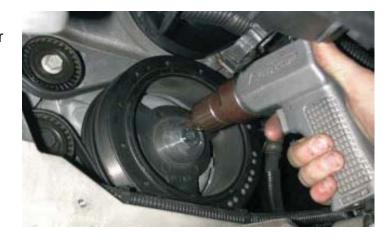
74. Using a 24mm socket, remove the large bolt and the drill guide from the engine.
