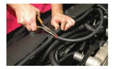
130. Loosely zip tie the hoses together, pass below the power steering reservoir and up toward the coolant vent pipe.
