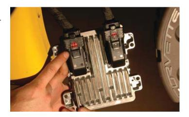
10. Remove the computer connectors carefully by pulling straight out.
