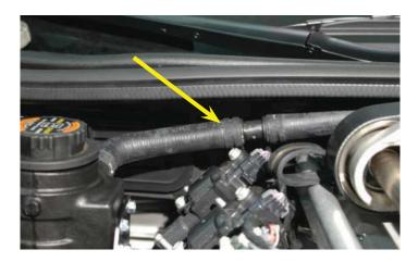
214. Cut 2" off the short end of one of the supplied ¾" x 4" x 36" elbow hoses. Install this short end onto the driver side barb of the supercharger intercooler using one of the supplied worm gear clamps. Route this hose over to the passenger side and forward between the reservoir and the coil brackets.
