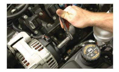
174. Connect the fuel line to the supercharger fuel rail manifold barb. Test the line by pulling firmly; you should not be able to remove the fuel line without using the fuel line removal tool.
