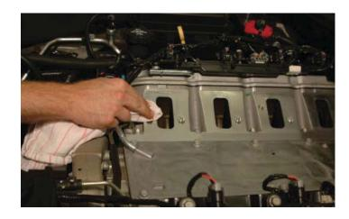
46. Cover the intake manifold ports with tape or clean rags to keep dirt and objects from entering the engine.
