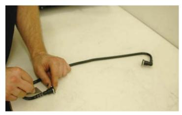
183. Connect the 90° elbow to one end of the supplied 5/16" hose. Use the supplied black spring clamp to secure the connection.
