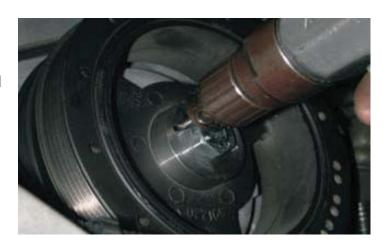
72. Using compressed air, blow the drill shavings out of the holes.
