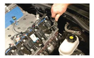
138. Remove the coil brackets for modification.
