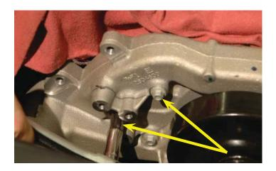
110. Use a die grinder, reciprocating saw, hacksaw, or what have you to cut off the two bosses shown level with the face of the surface of the boss from the removed bolts.
