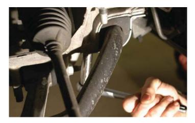
49. After removing the sway bolts, brackets and end link nuts, remove the sway bar and set it aside.
