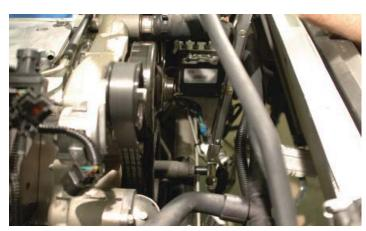
71. Using a small or angled 3/8" drill and the supplied drill bit, insert the drill into the guide holes and drill to the second step of the drill bit. (Make sure that you drill all the way to the second step.)
