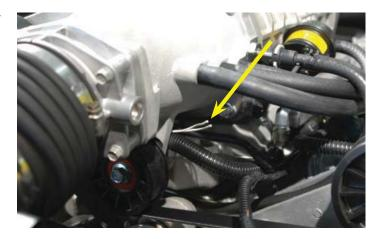
270. Connect the MAF plug extension to the MAF plug you installed earlier in the new air tube.
