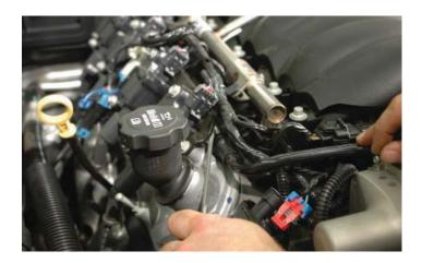
29. Disconnect the EVAP solenoid electrical connection.
