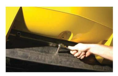
204. NOTE: If your vehicle had the soft rubber air deflector removed in step #194, this will be done at a later moment. If not, install the Heat Exchanger retaining bracket with the bolt removed in the previous step. Ensure that the foam pad is contacting the lower tank of the heat exchanger and tighten the bolt securely.
