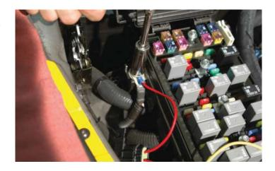
230. Zip tie the fuse holder to the hood release cable below the positive terminal of the fuse center as shown.
