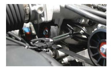
274. Replace the computer connectors in their original positions, making sure to lock them in place by pushing the grey levers towards the harness. Secure the connectors by inserting the red lock keys in position.
