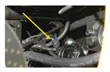
244. Inspect your coolant hoses carefully and add sections of the provided split loom to protect the hoses from any chaffing and rubbing on hard or sharp edges.
