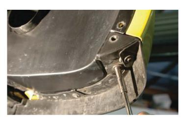
188. Remove the front driver side splash panel assembly from the vehicle. You will need to separate the pieces for re-assembly later.
