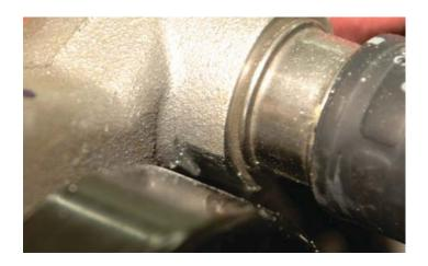
114. Install the new tensioner mounting bracket in the original location of the OEM unit with one original bolts and one countersunk Allen bolt. Torque the bolts to 40 ft-lbs; be sure to verify your torque wrench settings.
