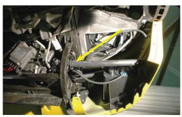
219. Cut 2" off the short end of the other supplied ¾" x 4" x 36" elbow hose and connect to the passenger side barb on the heat exchanger using a supplied spring clamp. Route the long end of the hose through the same hole the driver side hose you just installed used.
