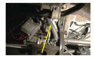
222. Cut the remaining end of the hose from the intercooler pump inlet barb to fit to the discharge barb on the intercooler reservoir. Clamp onto the barb using one of the supplied worm gear clamps.
