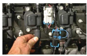
168. Before you tuck the wires of the injectors harness below the coil packs, remove the tape off the passenger side harness to about the center bolt of the coil pack. This is to free the MAP sensor plug from the harness where it will change direction and go to the rear of the supercharger.
