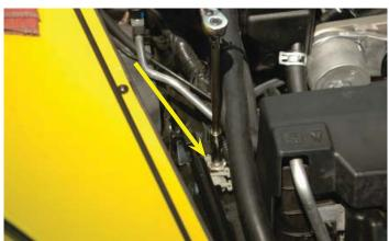
232. Route the black ground wire from the intercooler pump harness to the stud you just exposed and add the "eye" terminal to the ground, replace the nut and tighten with a 10mm wrench.
