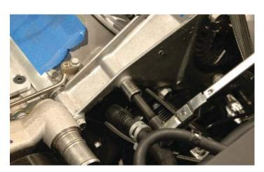
128. Remove the hose and clamp from the coolant vent "T" fitting.
