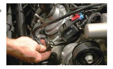
26. Release the vent tube at the top of the EVAP solenoid by pushing in on the release trigger.
