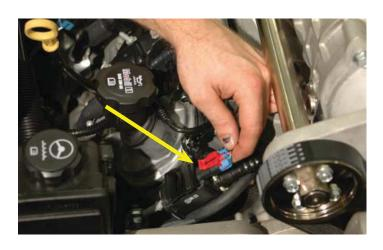
172. Remove these two alternator cable mounting clamps from the wire loom. The front clamp will remain in place and be utilized.
