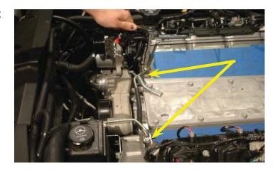
90. Install the new O-ring gaskets on the vent pipe blocks using some of the supplied Lubriplate lubricant to hold them in place.
