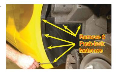
6. Remove the Push-lock fasteners by gently prying up on the center of the fastener and then removing the fastener completely.
