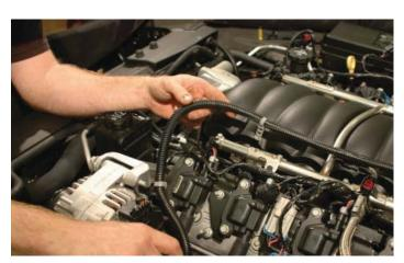
36. Free the battery cable from the intake manifold and lay it aside.
