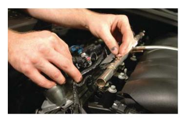
33. Disconnect the eight fuel injector connectors by pressing in on the release triggers and pulling the connectors free.
