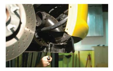
246. Attach the fender well splash shield, twisting to lock the brake cooling duct back into position and fasten using all the original hardware and locations. This includes push pin rivets and bolts.
