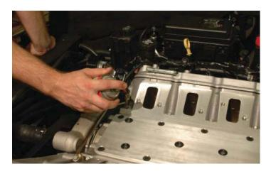
152. Carefully, set the supercharger assembly on the engine, line up the bolt holes with the holes in the cylinder heads. (Be careful of the one bolt located under the rear supercharger pulley on the passenger side as it protrudes and must be aligned first.)
