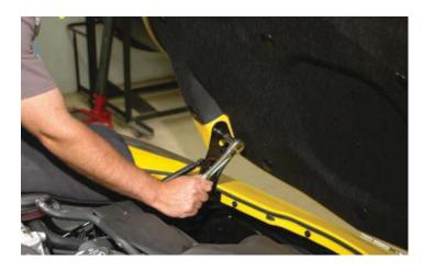
16. With a cool engine, open the petcock drain on the passenger side of the radiator and release the coolant into a clean drain pan for reuse later. Remove the radiator cap to vent the system. (Be careful not to remove the radiator cap if the engine is still hot.)
