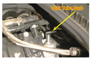
28. Disconnect the other end of the PCV tube that was removed from the air tube in step #21 which connects to the hose barb at the front of the passenger side valve cover. You may need to use a small screwdriver to release the clip lock which could be on the bottom.
