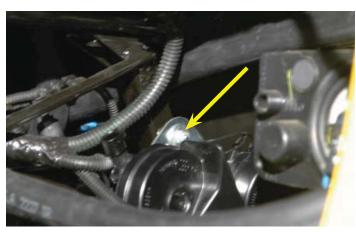
243. Reconnect the horn plug to the horn assembly.
