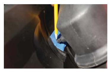
260. Remove the bellows and airbox, use an awl or center punch to mark through the tape onto the splash shield/air deflector.
