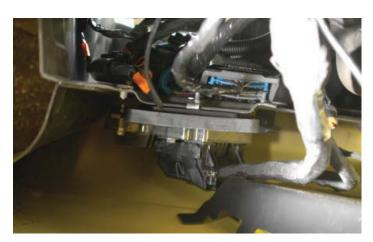
276. Reverse the steps, and re-install the plastic panel covering the ECM and TCM. This was removed in steps 5-7.
