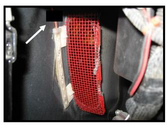
This car has cove screens over the openings but procedure is the same. Clean the area next to the opening with the supplied alcohol swabs.
