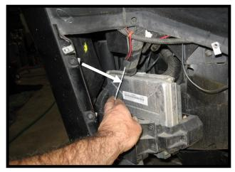
This shows where the coat hangar comes out in the passenger side cove area by the computer.
