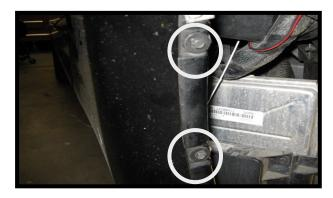
Remove these 2 x 7mm screws and remove the cove shield Now is a good time to paint the cove shields so they can dry.
