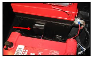
The control box can be mounted by the fuse box or anywhere convenient. Try to keep it away from heat.
