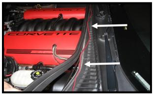
Next pull the cowl weaterstrip off by pulling it forward. Route the long led wire across the cowl to the drivers side hood latch area. You can also run the wires behind the engine away from exhaust.
