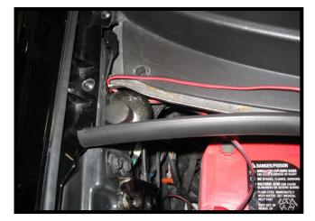
Now hide the wire under the cowl weather strip. Slip the weather strip over the wires being careful to not damage the wires. You may want to open up the weather strip to make it easier to slip over the wires. You can also tuck the wires behind the battery and engine as long as they don't hit anything that will burn them.
