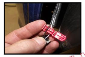
Insert one wire in the metal V of the connector and fold shut. Use a pair of pliers to make sure it atches shut. Repeat for both wires.
