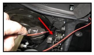
outside of the brake booster where you can pass the led strip into the fender cove area (red arrow). If you have trouble finding this area you can remove the lower splash shield in the next step and use a light to make it easier.
