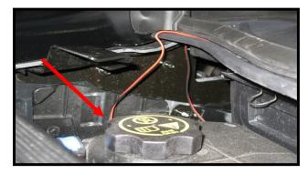
You can now test the lights before you complete the installation. Drop the shorter wire and led strip down into the fender cove area on the passenger side (red arrow)
