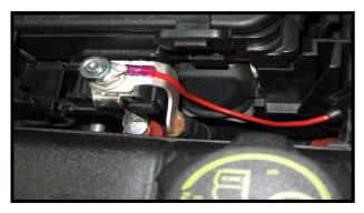
Route the red wire to the back of the fuse box and install it in this position and tighten. Close the cover.
