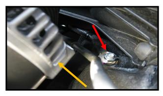
Locate the negative cable (red arrow) below and in front of the alternator (yellow arrow). Route the black wire from the control box and attach it to this cable with the provided nut. On Z cars you can use the bolt on the oil tank as a ground.
