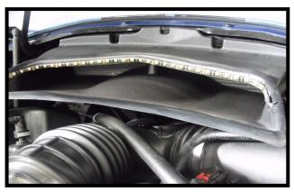
Open the hood and Center the hood vent led strip on the ducting as shown. Be sure the wiring comes out on the passenger side as shown in the next picture. Be sure to prep the mounting area with the adhesion promotor.
