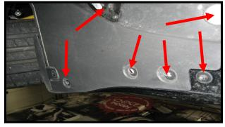
You can take this panel off to gain more access to the cove area. You will have to take this panel off or down a little if you are connecting the rear facia kit to the cove kit. Raise the vehicle up using the factory lift points and support with jack stands. Remove 4-7mm screws and 2-10mm screws. One 10mm screw is hidden in this picture (upper left arrow). Pull this panel back to gain access to the fender cove area to place the leds.
