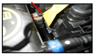
locate this tab on the back of the fuse box to release cover over positive cable (red arrow). Pry tab rearward to release and open cover over positive cable. This is where you attach the positive wire from the control box with the supplied nut.
