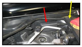
Open hood and place control box in this location (red arrow) in front of under hood fuse box (yellow arrow) or you can mount it under the cowl lip. Do not attach until installation is complete. The extra leads are for the hood vent leds.
