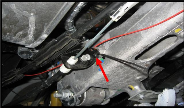
After installing the rear facia kit route the long lead with the wire connectors to the drivers side of the rear facia so the connectors will reach the rear facia led connectors. You can route the wires behind the E-brake cable mounts (red arrow) and secure with wire ties.
