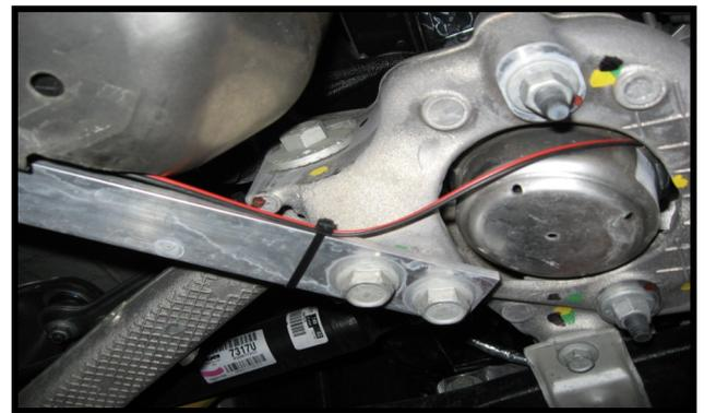
Feed the wire through this area and secure to the flat bar.
