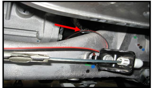
Red arrow shows suggested wire routing to get to the front of the vehicle. Go over the rear cradle then above the leaf spring
