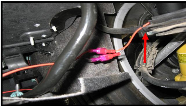
This shows the wires connected and wire tied to the E-brake cable (red arrow).
