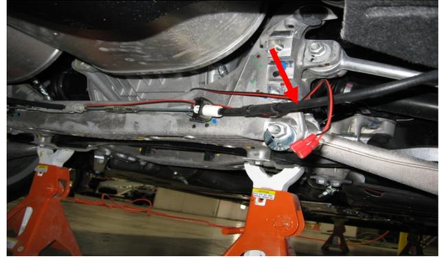
This shows the passenger side wire secured to the E-brake mount. Make sure the short lead with the connectors reaches the rear facia led wires. Once connected secure the wires to the E-brake cable or other brackets to keep away from exhaust.
