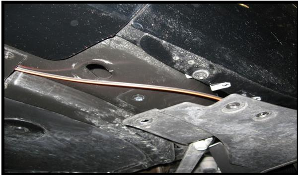
This shows the wire exiting the rocker panel and going to the cove area to be connected to the extra leads on the cove led kit.
