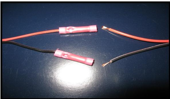
Strip 1/4" of the insulation off the ends of the wires, fold the wires to double their thickness for a better hold when crimping. Insert in the connectors and crimp tightly.
