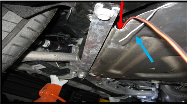
Route the wire inside this aluminum shield which should bring the wire to where the fishing wire came out (blue arrow).
