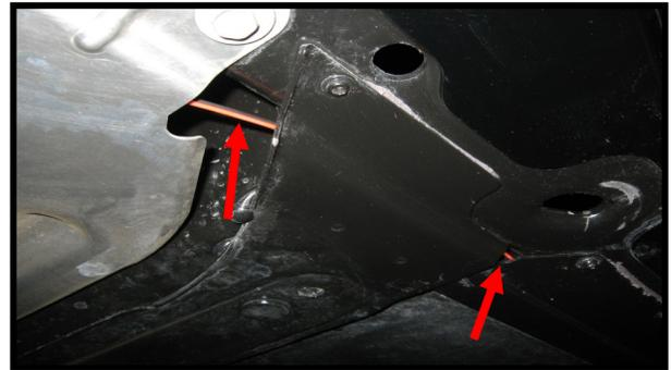
Tightly tape the wire to the end of the fishing wire and pull it through to the front of the vehicle.
