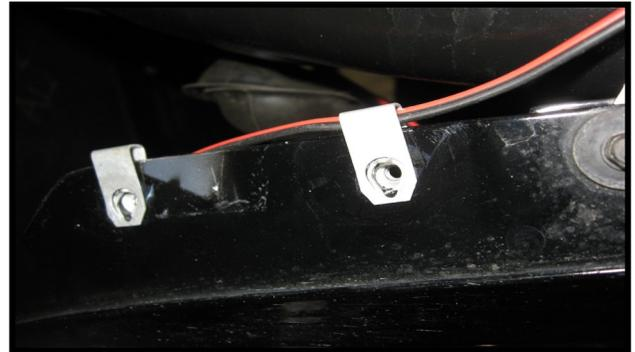
You can secure the wire by removing this clip and putting the wire in the end loop then re-install it.
