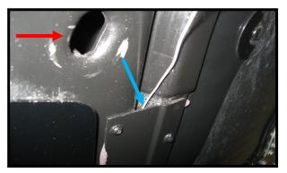
Place the car on jack stands to gain access to the underside of the car. Starting at the front, Locate this area just behind the front lifting hole (red arrow). Insert the stiff wire into the opening (blue arrow) and slide it through to the rear of the car. Make sure the wire is straight so it doesn't catch on anything.
