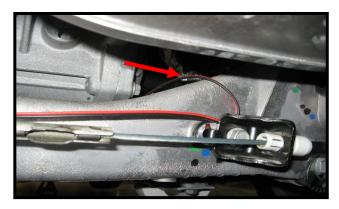
Red arrow shows suggested wire routing to get to the front of the vehicle. Go over the rear cradle then above the leaf spring
