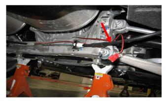
This shows the passenger side wire secured to the E-brake mount. Make sure the short lead with the connectors reaches the rear facia led wires. Once connected secure the wires to the E-brake cable or other brackets to keep away from exhaust.
