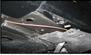
This shows the wire exiting the rocker panel and going to the cove area to be connected to the extra leads on the cove led kit.
