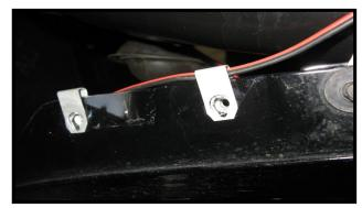
You can secure the wire by removing this clip and putting the wire in the end loop then re-install it.
