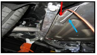
Route the wire inside this aluminum shield which should bring the wire to where the fishing wire came out (blue arrow).
