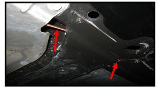
Tightly tape the wire to the end of the fishing wire and pull it through to the front of the vehicle.
