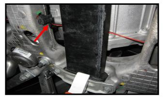
This shows the wire going over the leaf spring. You can secure the wire to the line at the red arrow.
