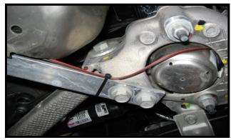
Feed the wire through this area and secure to the flat bar.
