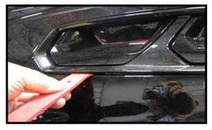
This shows the mounting tabs you are trying to release. There are 3 on top, 4 on the bottom and 2 on each side. Always pull out on the bezel as you are releasing the tabs. You can use a shop towel to protect the paint.
