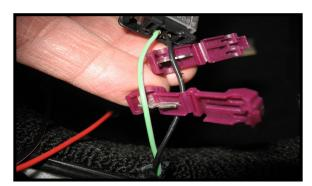
Place one wire in each of the supplied quick tap connectors, fold shut and close with pliers until they latch. The wires you see will be purple or brown and black.
