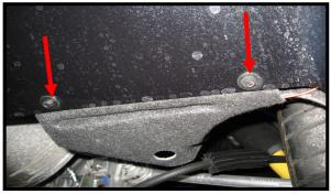
You can also remove these two 7mm screws for better access for routing the wires. Follow the next steps if you are connecting to the side marker lights so these leds come on with the lights. If you are connecting them to our front fender cove lighting kit you will need to purchase our under car wiring kit to connect the rear fascia to the extra leads on the fender cove lighting kit.
