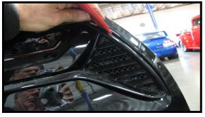
There are 2 retaining tabs on each side. You can use a hooked tool to pull out while you release the tabs. Once the bezel is removed drop the led wires down to the rear side marker connectors you previously disconnected.
