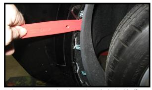
Using the panel removal tool, pry the splash shield off. It pops off easily.
