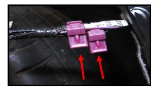
Now plug in the led wires into the back of the quick tap connectors. drivers side: Plug red led wire into purple wire, black to black. Passenger side: Plug red led wire into brown wire, black to black. Don't forget to plug the connectors back into the rear markers before you move on.
