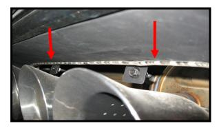
This shows where to mount the exhaust led strip. Clean mounting area with alcohol pad and prep with adhesion promoter before peeling the backing and mounting the strip. Wire tie all the wires up and away from the exhaust.
