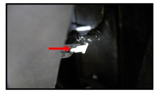
This shows the rear side marker connector. Slide the white tab as shown to unlock the connector from the housing. Pull the connector out so you can wire the leds. If you can't pull the wires out far enough to wire, there are additional harness retainers you can release after removing the tail light bezel.
