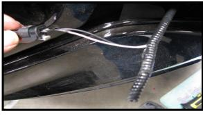
Now split the side marker harness open and pull the wires out for access.
