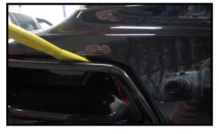
Carefully insert the panel removal tool between the taillight bezel and the rear fascia, pry down while pulling the bezel out. Work your way around the bezel releasing the tabs holding the bezel In place. See next pictures.
