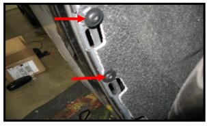
Remove these #15 torx screws behind the splash shield for access to the rear side marker connector.
