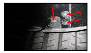
Raise rear of vehicle and support with jack stands. Locate these three 7mm screws behind the rear wheels and remove on both sides of car.
