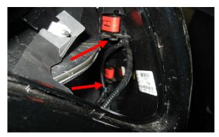
Looking through the taillight opening there are 2 places that the wire harness is connected to the body (red arrows). Pry the retainers out so you can position the wire harness to tap into the wires. You can pull it out of the taillight opening or access the harness through the fender opening behind the rear
