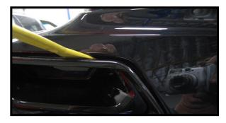
Carefully insert the panel removal tool between the taillight bezel and the rear facia, pry down while pulling the bezel out. Work you way around the bezel releasing the tabs holding the bezel In place.
