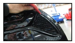
There are 3 tabs on top, 4 on the bottom and 2 retaining tabs on each side.
