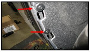
Remove these #15 torx screws behind the splash shield for access to the rear side marker connector. Pull back the liner and feed the led wires up to this area and pull through.
