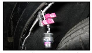
Pull the connector out as far as you can, split the wire loom and separate the wire to install the connectors. If you cannot get the connector out far enough follow the steps on page 2
