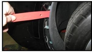
Using the panel removal tool, pry the splash shield off. It pops off easily.
