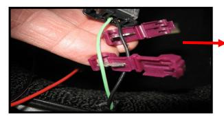
Using the supplied connectors place 1 wire in each metal clip and fold the connector closed until it clicks shut. You may need to use pliers. Wire colors are: drivers side: purple is positive. Black is negative Passenger side: brown is positive, black in negative.
