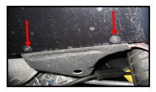
You can remove this panel if you need more access to feed the wires up to the side markers. Remove 2 #15 torx screws.
