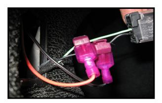
Route the led wires up to the installed connectors and plug them in to the back of the connectors.
